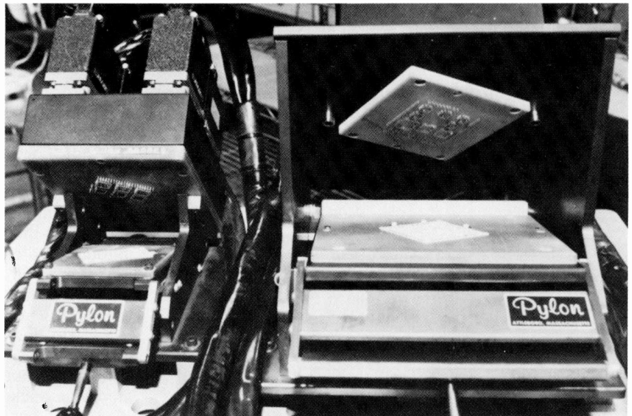
Fig. 4. Custom probe fixtures are ideally suited for testing circuits in medium and high quantity, and can handle counts of several thousand probes.
