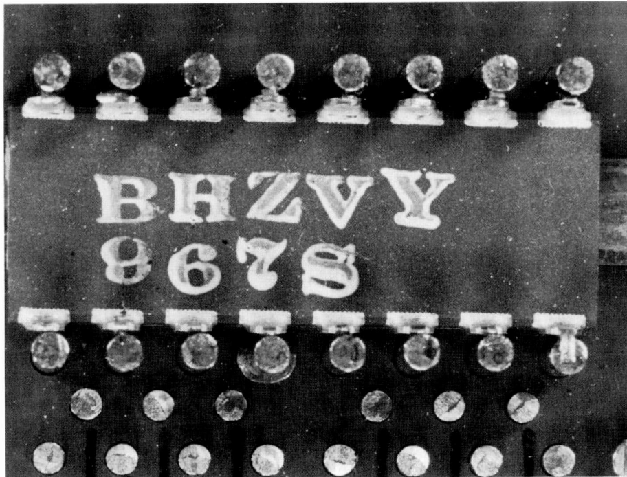
Fig. 8. Top view of integrated circuit (dual-in-line package) illustrates how leads are pincer-welded to button of buttonhead pins.
