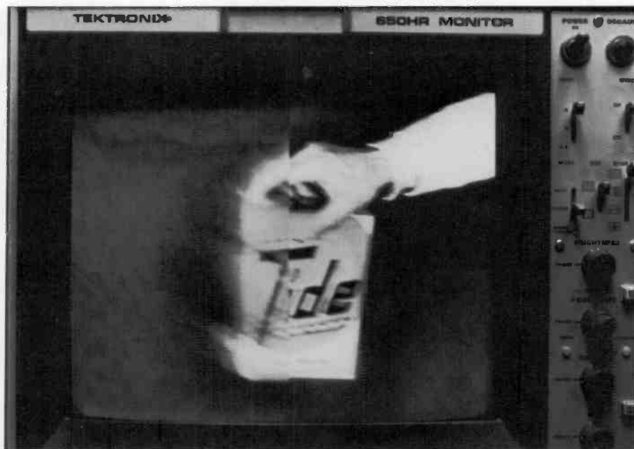
Fig. 6. Split-screen photo of TV monitor comparing superior lag characteristics of RCA broadcast CCD camera. Saticon tube camera is on left, RCA CCD camera is on right.
