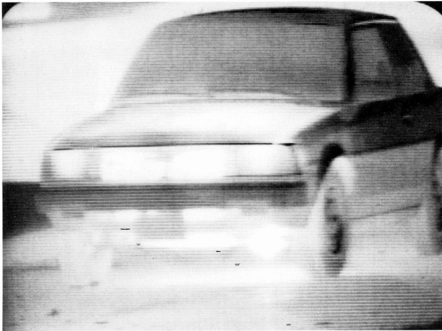
Fig. 8. TV monitor photo of night imagery taken with 160 \times 244 Schottky barrier-IRCCD imager developed at RCA Laboratories.
