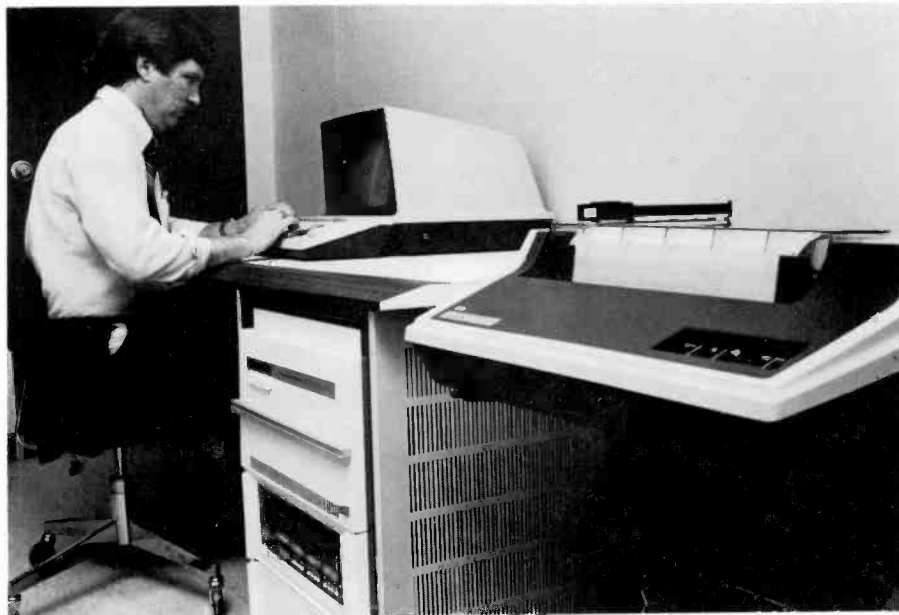
Fig. 3. A Hekimian Test System allows remote, after-hours testing (by Pete Byrnes, Technician) of intermachine trunks and other voice-grade services. Trouble tickets are issued to the CSC on suspect circuits for trouble verification and resolution.
