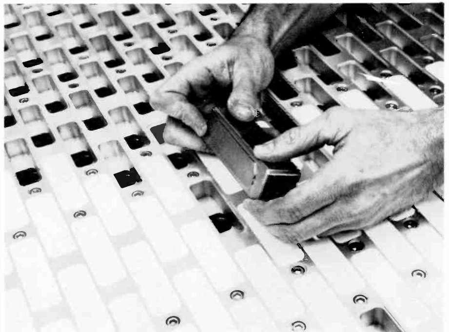
Fig. 4. Alumina windows are carefully placed by hand in the face of a metallic antenna mockup. Robotics are planned for the actual assembly.
