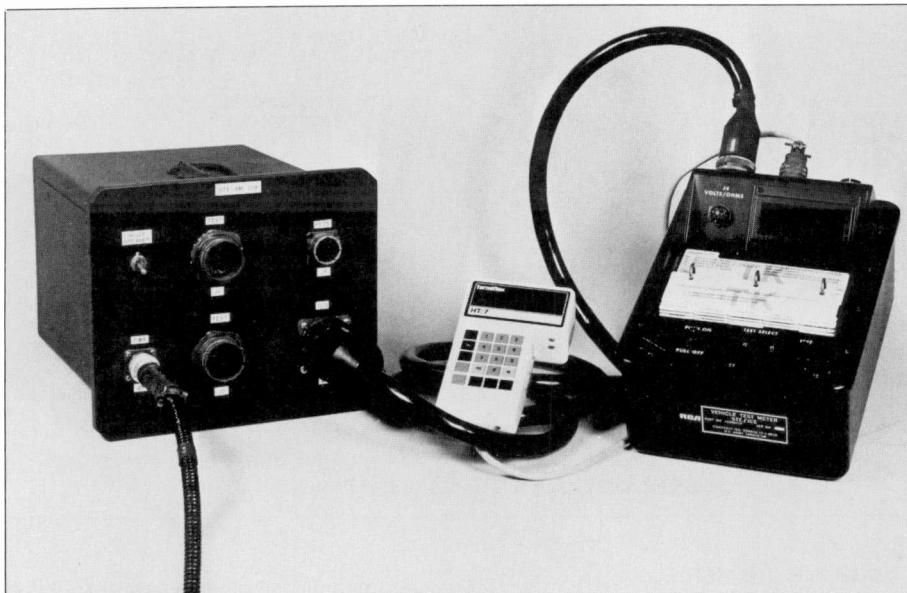
Fig. 1. Simplified Test Equipment for the Army's Abrams M1 tank and Bradley Fighting Vehicle System (STE-M1/FVS). The STE-M1/FVS is three separate units—the VTM (right), the SETCOM (middle), and the CIB (left). The VTM, Vehicle Test Meter, the main controller of the system, handles input from and output to the user and controls the analog measurement system. The SETCOM, set communicator, is a small hand-held terminal with 18 input keys and two 20-character output lines. This is used to enter the test number, guide the user through a diagnostic test, output fault messages, and to query the user for information. The CIB, Controllable Interface Box, provides the VTM with a 256-channel analog measurement system, which contains its own computer. The VTM communicates through a serial link to the CIB and commands the CIB to make a measurement and return the results.
