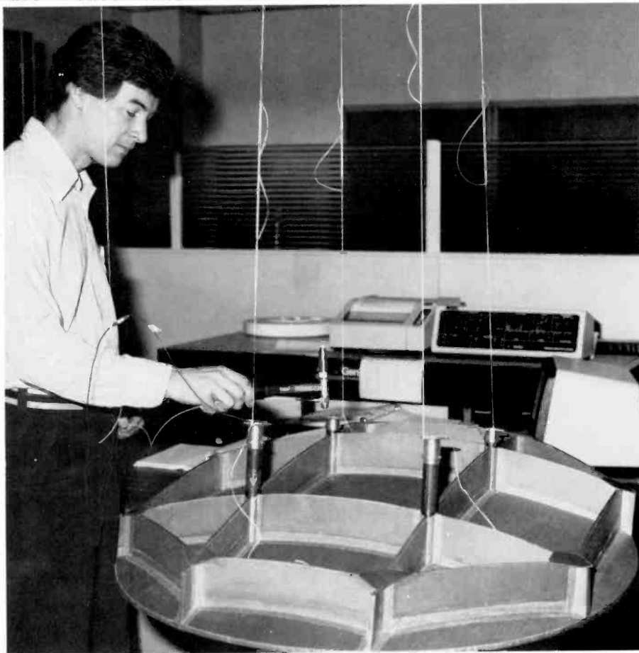
Carl Voorhees, Senior Member Technical Staff at Astro, checks the setup for modal testing of a K-band reflector.
