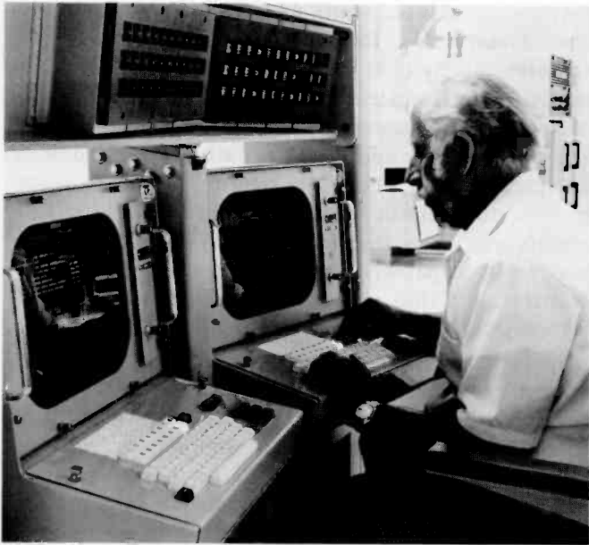
Fig. 2. Lawrence Schulman, Test Specialist with the AEGIS group of ICSS, mans the test monitor central console of the Operational Readiness Test System. Under computer program control, the system provides status assessment, maintenance control, and testing of radar, fire control, and other elements of AEGIS.
