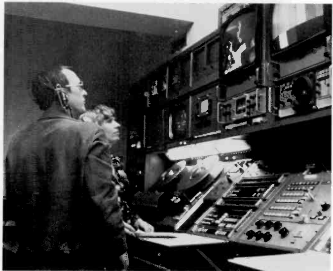
Fig. 12. An edit bay at NBC, Burbank, California. To the right of the edit system is a video switcher with dissolve-and-wipe capability, and a small audio mixer. These added devices expanded the signal manipulation capabilities in parallel with the increased sophistication of the editor. (Courtesy EECO)
