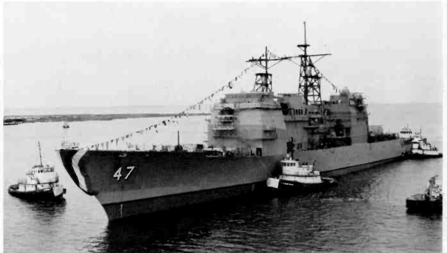
The "float off." Tugs move the Ticonderoga to its outfitting berth following submergence of the special launch pontoon in the Pascagoula River.
