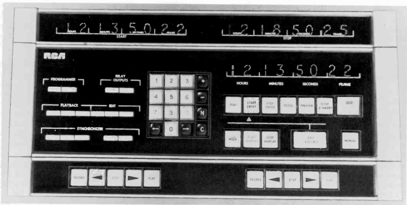
Fig. 11. TCE-100 edit controller. This system included three code read-outs; edit controls on the main input panel, including a keypad for timecode entry; and a transport control panel.
