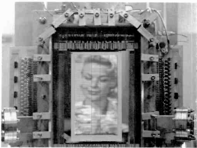
Fig. 9 (a). Off-the-air video displayed on a 12.5-cm x 25-cm (5 in. x 10 in.) black-and-white modular guided-beam display. The displayed image is only 1/25th of the total picture for a 1.27 m (50 in.) diagonal TV.
