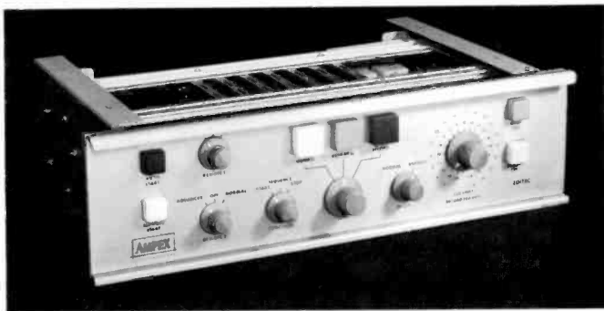
Fig. 8. Early model of the Editec programmer. Later versions included a video only mode, animation controls, and secondary cue provisions. (Courtesy Ampex Corp.)
