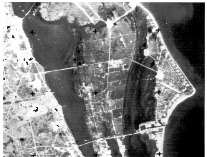
Fig. 9 Resolution of space images has improved. These images of the Cape Canaveral area were both taken by return-beam vidicon tv cameras. For Landsat 3, the Landsat 1 camera was modified so that it covered half the distance at twice the resolution. Linear resolution improved from 80 meters to 40 meters, with a consequent 4X improvement in area resolution. (NASA photo.)
