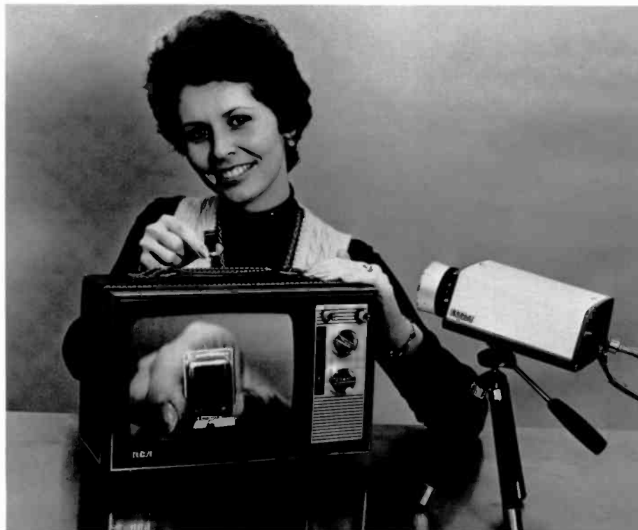
7. CCD image sensor shown on the tv screen is the heart of the tubeless tv camera developed by Electro-Optics.
