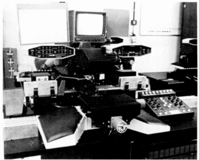
Fig. 7. The die-attach machine, a fully automatic system with pattern-recognition, adhesive-epoxy dispensing, frame-handling, and die pick/place features.
