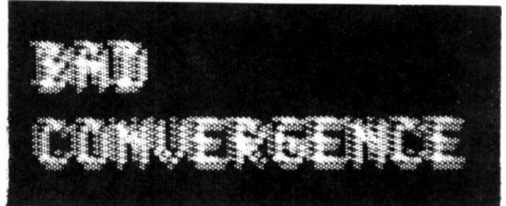
Fig. 11. Example of good and bad convergence. RCA 13V high-resolution display tube. All three guns on.
