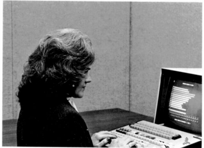
Fig. 2. A data-display CRT in a typical application. The CRT is used with keyboard, viewed from arm's-length distance.
