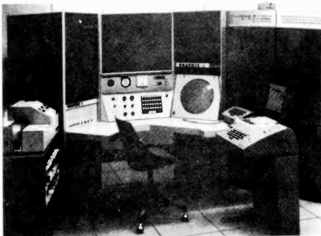
Fig. 8. The Graphic 1 Console System, developed at Bell Laboratories. Musical passages can be described in graphical notation by drawing on the CRT with a light pen. (From Music by Computers , John Wiley & Sons, Inc., 1969.)
