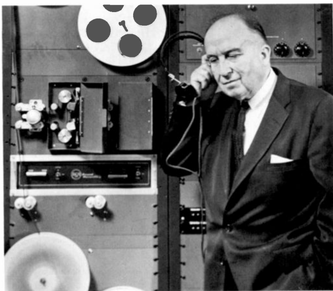
Fig. 1. Dr. Harry F. Olson in 1963 with the RCA Mark II synthesizer. This machine became popular with composers because it could be easily programmed, using paper tape, to produce analog sound sequences.
