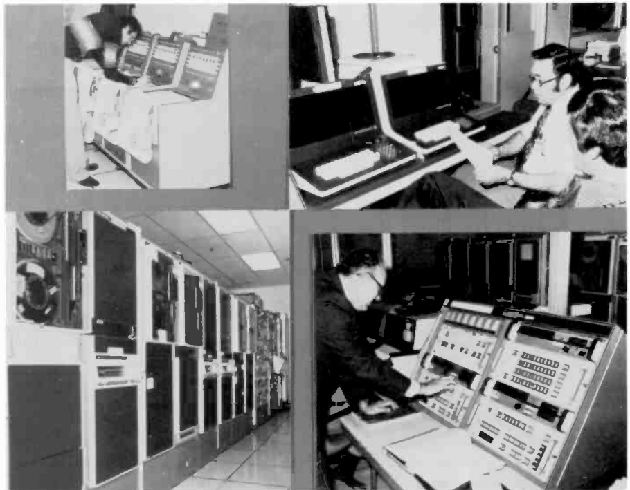
Fig. 6. TIROS-N Aerospace Ground Equipment (NAGE). Three Data General Eclipse computers are used in the automated test equipment to functionally test the entire TIROS weather satellite in 72 hours.
