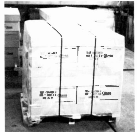
Humidity testing for Brazil: 16V tubes covered with large poly bag. Picture was taken at the Humidity Test Chamber in Camden.
