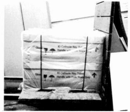
Incline impact test of 16V 90° tubes at Camden Packaging Lab. Four impacts per package exceed the expected real-life occurrence in truckload shipments.
