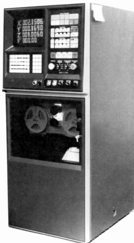
The Machine Control Unit interprets the NC program instruction and sends signals to cause the desired function to occur. This could be anything from causing a tool movement to turning on the coolant.
