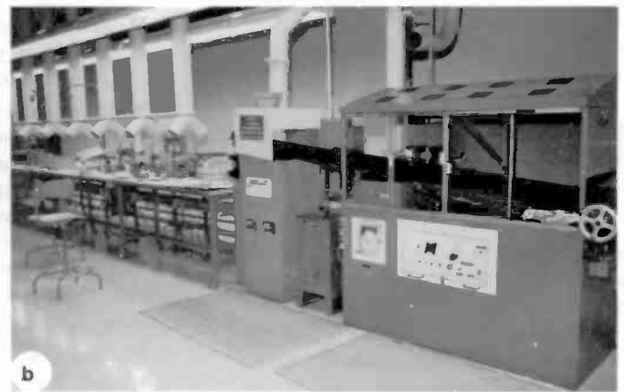
Fig. 3. The basic facility consists of (a) Man-U-Sert Inserting machine, and (b) bidirectional wave-soldering system.
