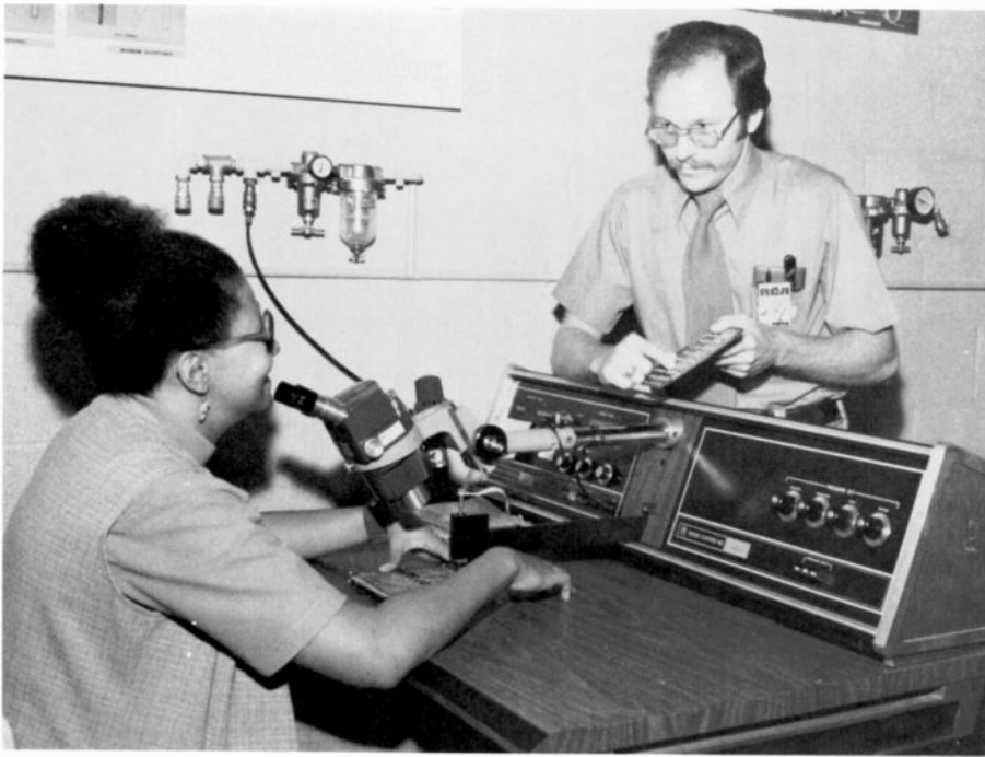
Fig. 3. Tape-controlled backplane-wire-welding station. Integrated circuit interconnection wire networks are welded using a tape-controlled weld station.
