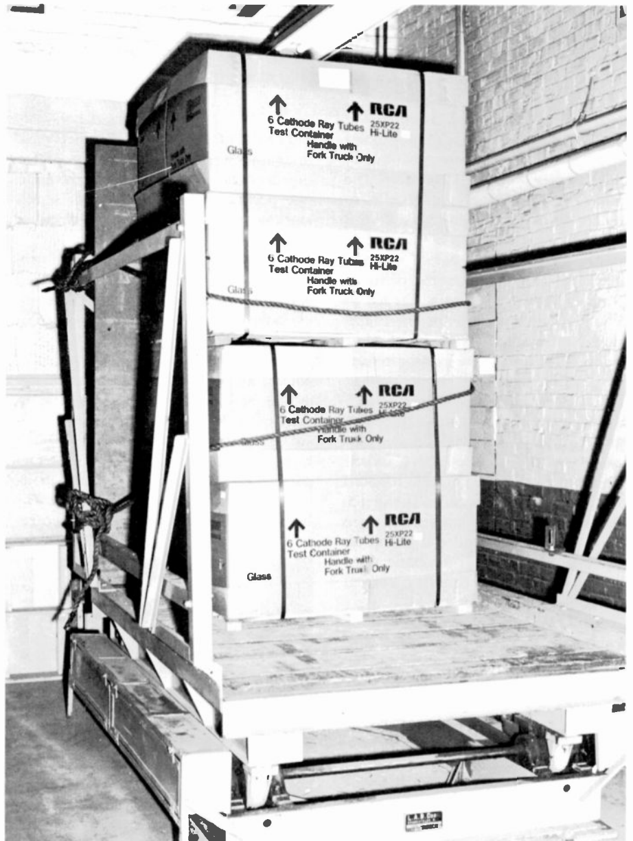
Vibration testing of two double pallet loads of 25V 90° tubes at Camden.
