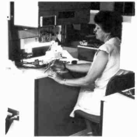
Fig. 10 Automatic test equipment (ATE). This computer-based tester is one of several that align and test the signal boards of the VideoDisc player. This unit uses computer-controlled motor-driven alignment tools to align the signal-board circuits. It also contains a built-in signal system to provide the test signals used during alignment and test.
