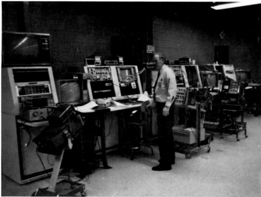
Fig. 5. Manual and automatic test equipment were used for testing PC boards, electronic assemblies and the player.
