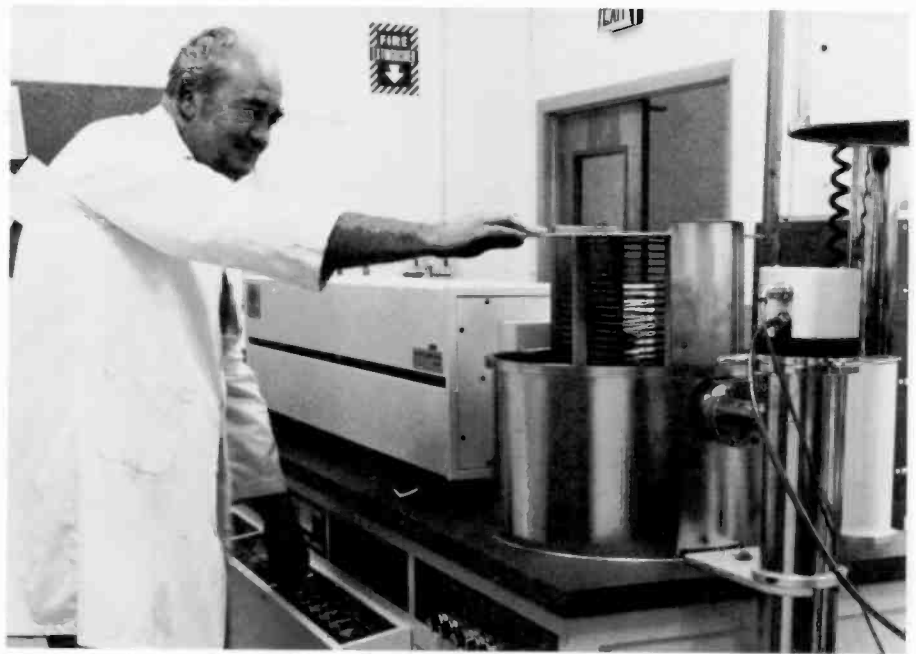
Fig. 2. Parylene-coating equipment with coating fixtures being inserted.
