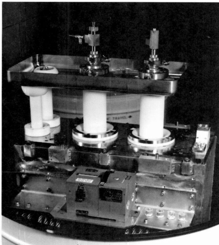
Fig. 7. Complete NBSM mounted in shipping container. Note that the coils of the helical isolators are visible just inside the front edge of the steel drum. Accelerometers (box and short cylinders in foreground) as well as high-voltage insulators (white cylinders) are also visible.
