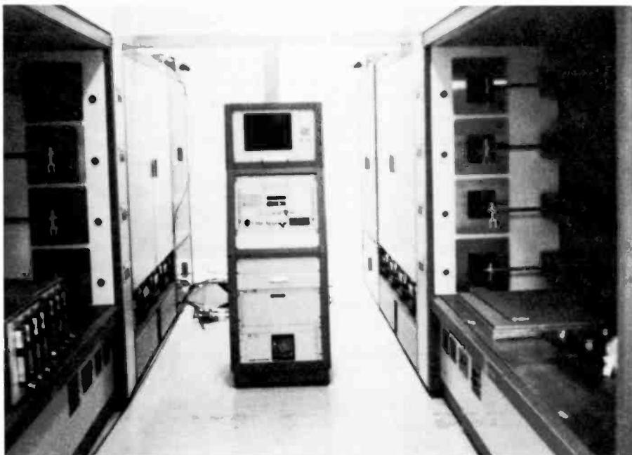
Diffusion-furnace complex manufactured by Thermco , showing eight diffusion tubes for wafers up to 100-mm. in diameter. Each tube can be individually programmed with its own multi-step sequence for oxidations, diffusions, depositions, anneals, and so on. Programmable parameters include: temperature (400-1200°C.), time for each step, gasses for each step, ramp rates entering and leaving the tube, and boat position while in the tube.
