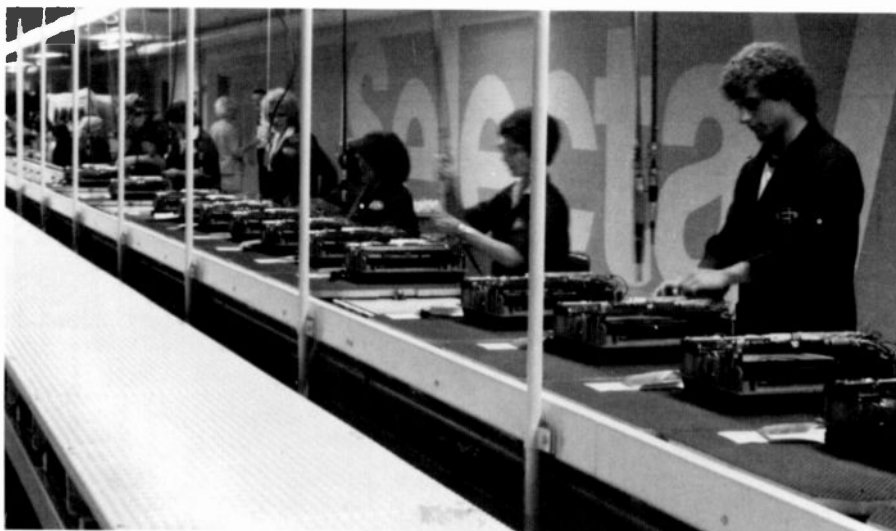
Fig. 7. Assembly line for the VideoDisc player. As a player progresses along this assembly line, it is gradually assembled by the many operators stationed along the line. Each operator, in turn, assembles one or more components (for example, the turntable) or subassemblies (for example, control-board assembly). At the end of the assembly operation, the test operation begins. Finally, before the player is transported to packing, the quality evaluation is performed.
