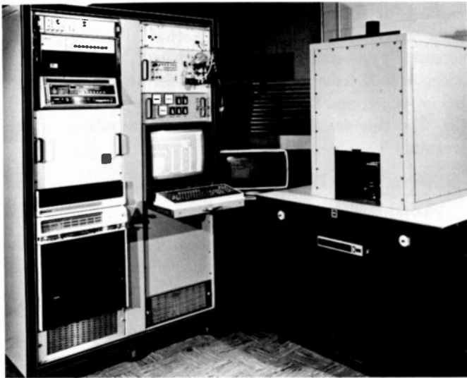
Fig. 6. AIME system. The system uses standard commercial video equipment to reduce costs and simplify maintenance.
