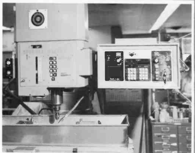
Fig. 6. Spindle Wizard™ numerical mill. The milling machine program is automatically loaded into the milling machine controller (shown at right) from the Tektronix 4051.
