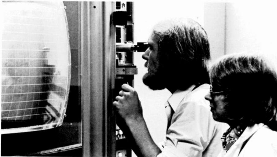
Technicians M. Grote and K. Sturlangson measuring yoke performance on TTL-designed test stand.
