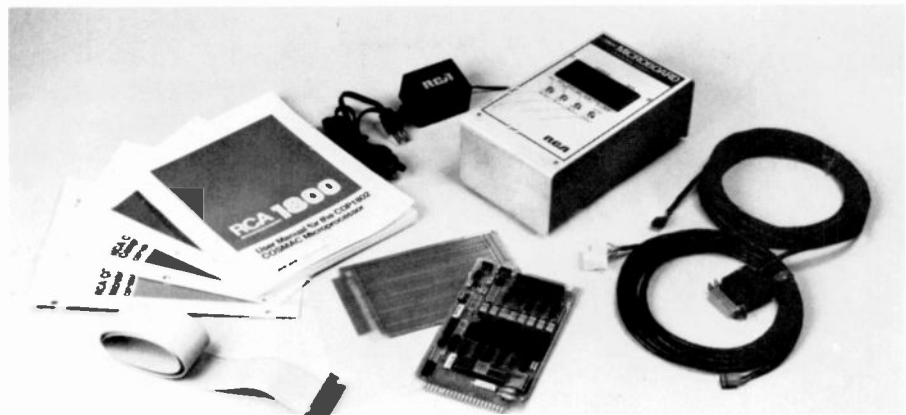
Fig. 2. The prototype kit allows the designer to design with CMOS Microboards with a minimum investment.
