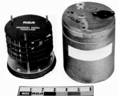
Fig. 5. Brassboard for acoustic micro-signal processor.
