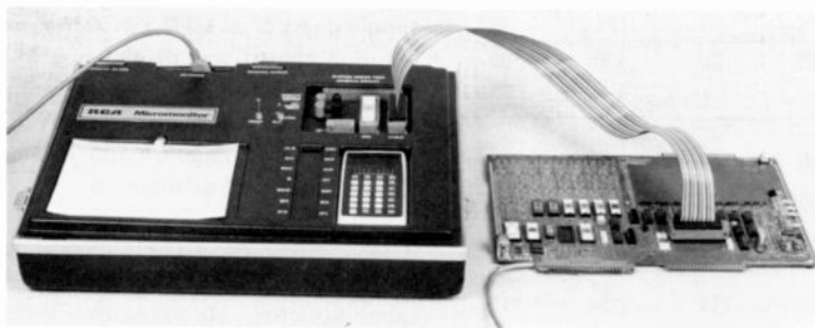
Fig. 4. The Micromonitor provides in-circuit emulation as well as debug capability.
