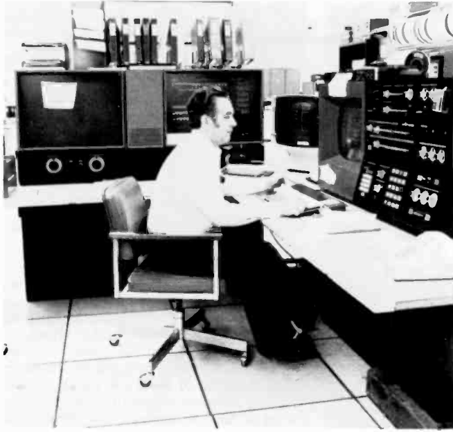
Fig. 1. IBM 370/168 computer system console and field engineering panel. The operator is shown viewing the tube on which system messages are displayed for his action. The operator is responsible for communicating with the system and performing duties which neither hardware nor software can provide.
