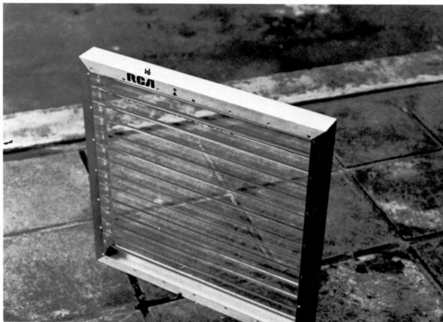
Fig. 1. Large strips of the piezoelectric polymer PVF 2 were used in this multi-element venetian-blind-like array.
