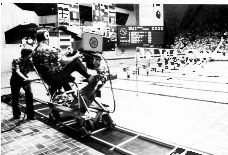
Fig. 4. Broadcast systems provided 17 TR-600 quadruplex video tape recorders, 5 TK-28 Telecine chains, 38 live color TV cameras, and 18 Video IV character generators to support the Montreal Olympic coverage.
