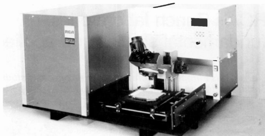
Fig. 2. Automated optical linewidth-measuring setup now in use at the Solid State Division.
