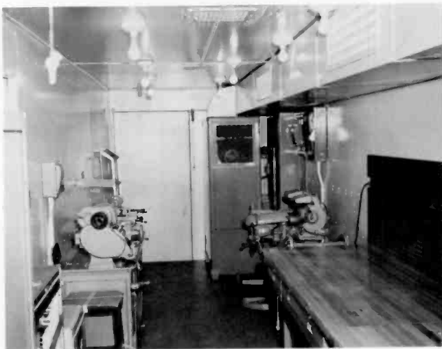
Fig. 3. This typical mobile overhaul van contains equipment and facilities for complete on-site overhaul of an instrumentation radar system.
