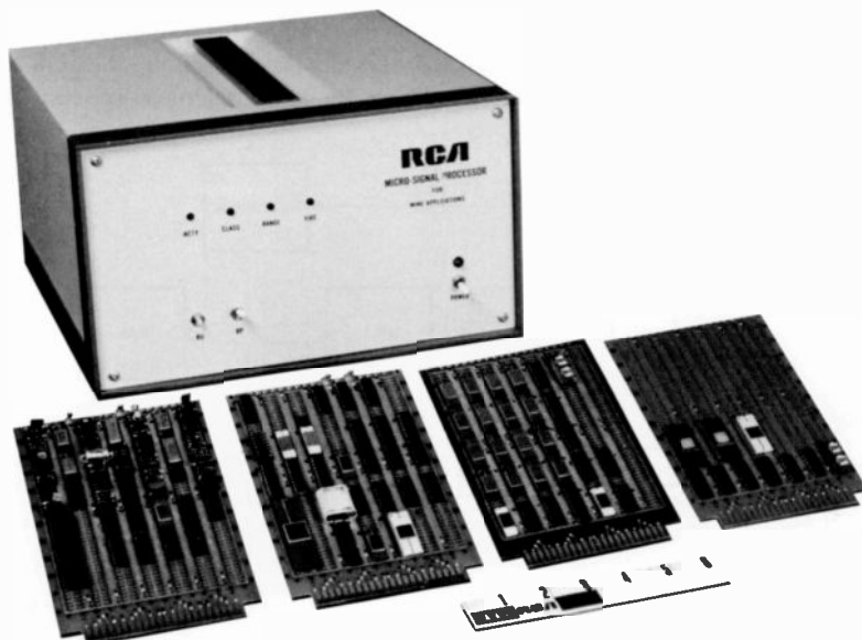
Fig. 4. Typical brassboard micro-signal processor for mine fuzing.
