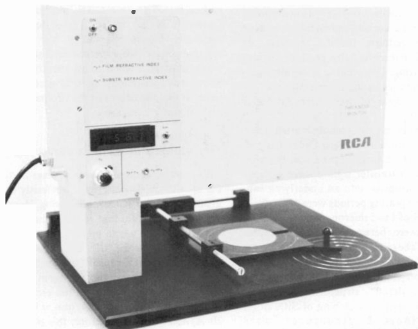
Fig. 5. Film-thickness monitor determines the thickness of a sample in seconds.
