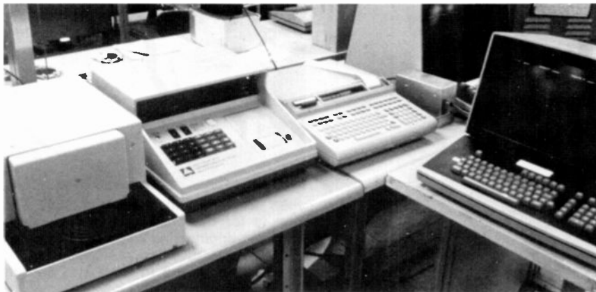
Fig. 6. Four point V/I probe subsystem. The probe is at left with its controller at center followed by the HP 9825 microprocessor and video terminal. This subsystem gathers resistivity data from prescribed positions on each wafer following a prescribed sampling plan.
