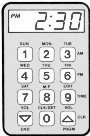
Fig. 2. Each programming command begins by pushing the start button and ends by pushing the end button.
