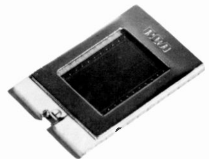
Fig. 12 Silicon imaging device intended primarily for use in generating standard-interfaced 525-line television pictures. This self-scanned device uses an array of charge-coupled device (CCD) shift registers for photosensing and readout. The device contains 512 vertical x 320 horizontal pixels (163,840 picture elements); chip size is only 500 by 750 mils.
