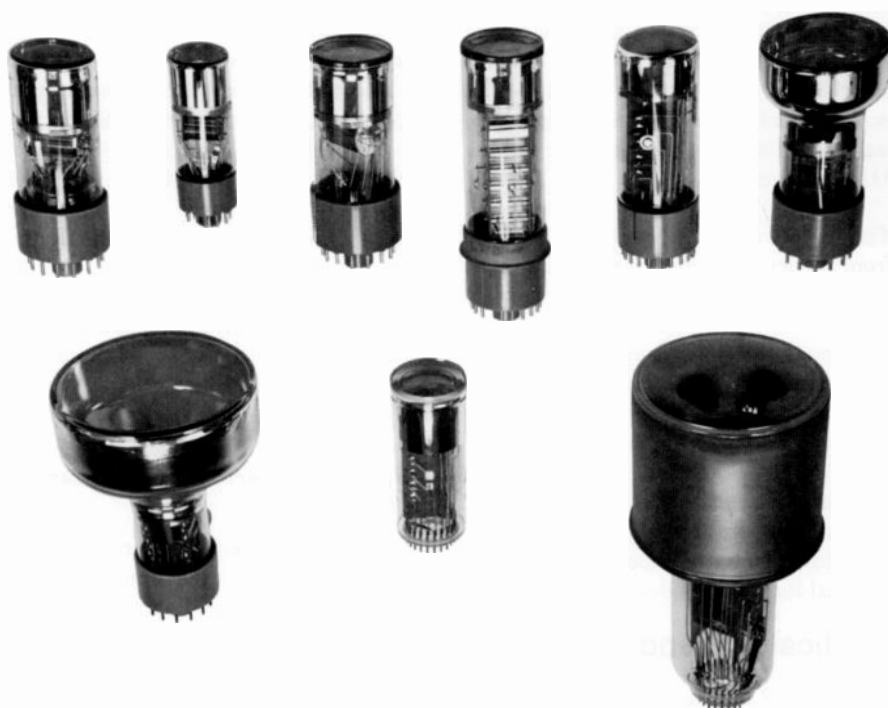
Fig. 10 Scintillation counting stimulated the development of several photomultiplier types. Left to right (starting on top) are the 5819, probably the first tube designed specifically for scintillation counting; the 6199, a smaller tube used by early uranium prospectors and also placed aboard a satellite by Dr. Van Allen and used to discover the radiation belts that now bear his name; the 6342A, which has a flat faceplate to provide an easier interface with the crystal; the 6810A, a 14-stage linear dynode tube for higher gain and less feedback between photocathode and collector (the circular arrangement is limited to 10 stages and the photocathode and anode are close to each other); the 7850, with improved electron optics for higher speeds needed to time certain nuclear events; the 8054, which handles larger crystals (about 3 inches) for better absorption of high-energy gamma rays; the 8055, which accommodates 5-inch crystals and contains RCA's "venetian blind" optics; the 8575, an improved 7850 with a flat faceplate; and the 8854, developed for the AEC for use in high speed measurements with plastic scintillators.
