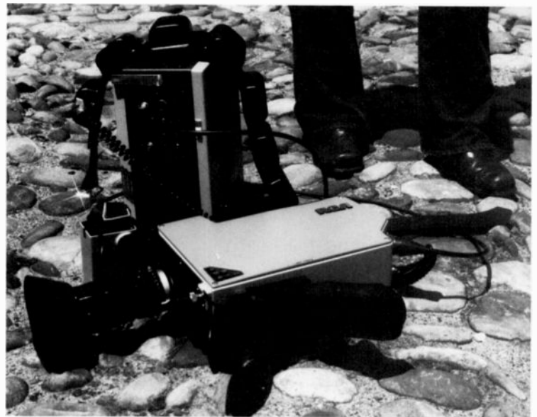
Fig. 3 TK-76 system consists of the camera and video tape recorder, which are tied together with an "umbilical" cord. Battery belt weighs only five pounds.
