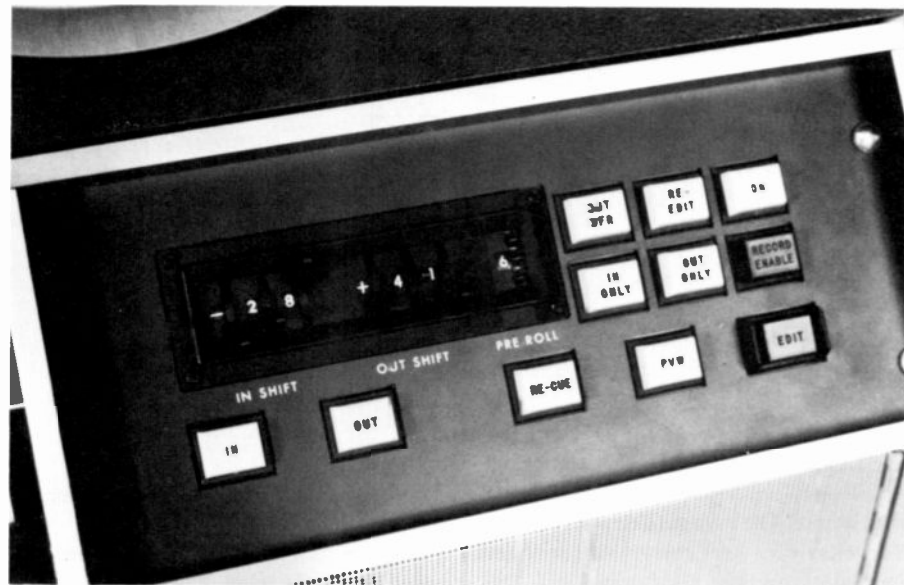
Fig. 6 SE-1 system (control panel shown here) is simpler than AE-600 system. It uses control-track signal on video tape, rather than a time-code signal.
