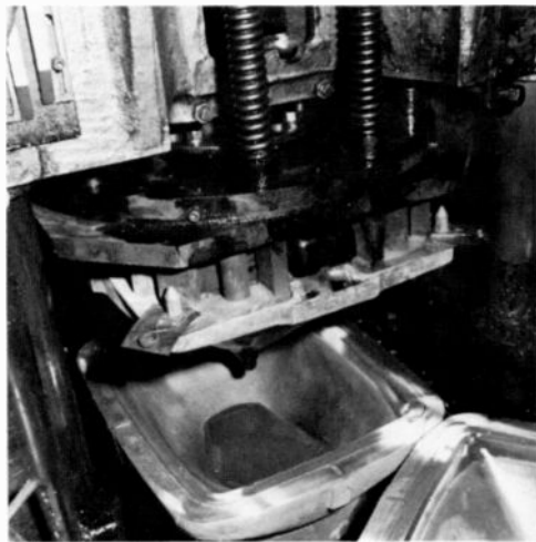
7. Hot glass in funnel mold.
