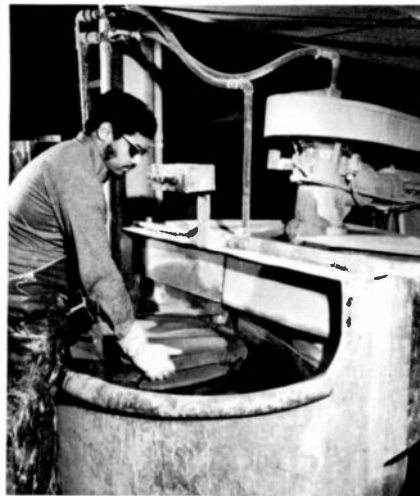
11. Polishing the outside surface of the panel.
