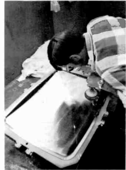
20. The mold surfaces are carefully polished after machining.
