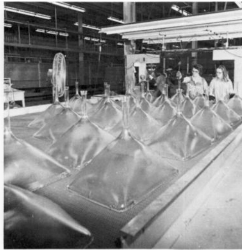
15. Parts are inspected after being cooled in a lehr oven.
