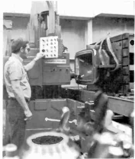
19. New mold equipment is prepared by N/C machining.
