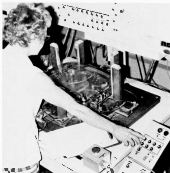
Stud-plane-to-contour gage in the gage room. Manual entry box is on the right side of the gage.
