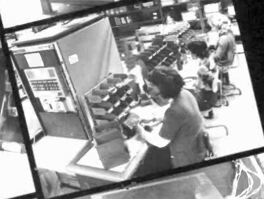
Below: power-transistor test console in final stages of checkout prior to installation on factory floor.
