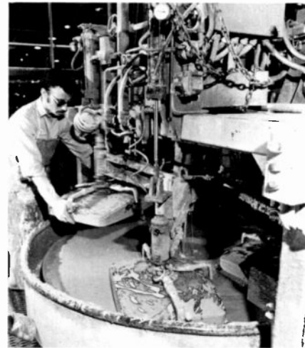
12. The sealing edge must be ground flat.
