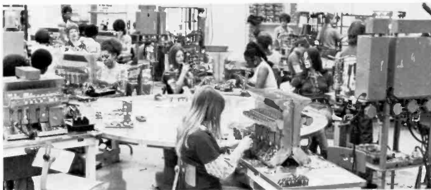
Various parts for the electron gun mount are assembled with a special fixture around a revolving work table.
