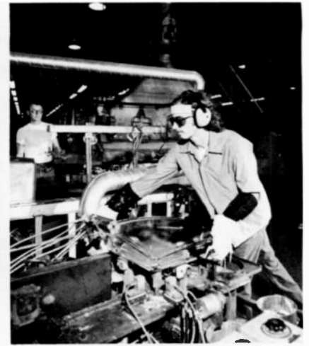
9. Metal pins are sealed into the sidewalls of the hot panel.
