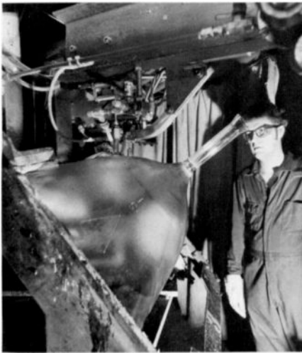
14. A metal button is sealed into the funnel sidewall.
