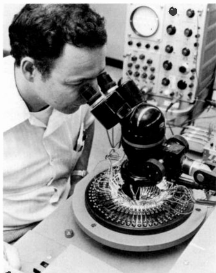
Above left: An array of precisely adjusted probes making contact with a COS/MOS integrated circuit on a three inch wafer. Each contact area on the I.C. is .004" square. Above right: Mary Lysy of COS/MOS Test Engineering using the off-line computer system with video keyboard to edit a test routine. This system is also used to translate written routines into test system language and to simulate the operation of the test routines.
