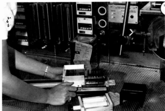
Fig. 5 — Furnace boat loading using transfer system.
