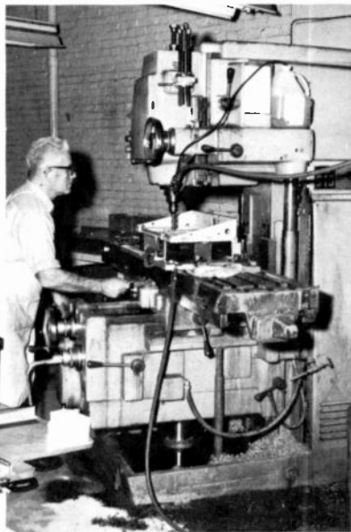
Above: vertical milling machine. Above right: horizontal automatic wire-wrap equipment.
