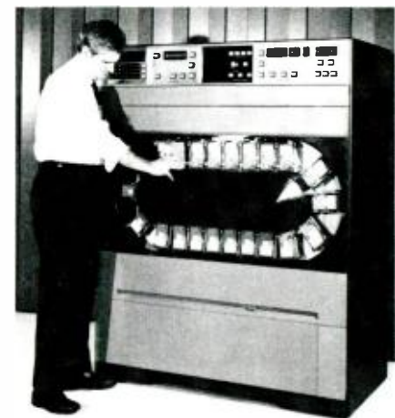
Fig. 4 — TCR-100 wideband mass data storage system. Each fully automatic cartridge equipment stores 8.8 \times 10^{12} bits of digital data (or an equivalent amount of analog data). Maximum access time is 25 seconds. These equipments can be "stacked" to provide an even larger data storage/retrieval capability.
