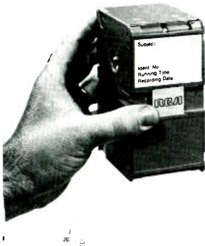
Fig. 5 — This cartridge stores ten complete ERTS frames with zero data reformatting. It stores easily and protects the tape from dust, dirt, handling abuses and other physical damage. Tape is good for several hundred passes due to rear side tape handling.
