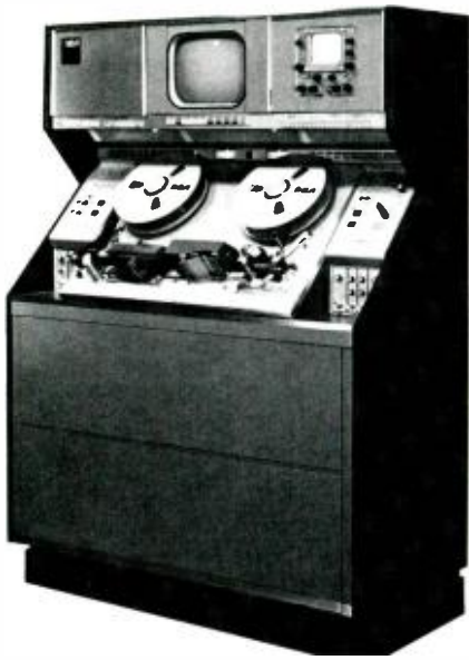
Fig. 3a — TR70-CVR-3E Recorder/Reproducer. This modified tv broadcast recorder allows either 15-Mb/s digital or 7.5-MHz analog instrumentation recording. Either multispectral-scanner (MSS) or return-beam-vidicon (REV) data from ERTS may be stored. The TR70 combines broadcast equipment production base with its inherent standardization, and advanced digital-analog processing techniques.
