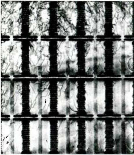
Fig. 3 — Projection topograph of silicon wafer showing dislocations introduced around the devices by the diffusion process.
