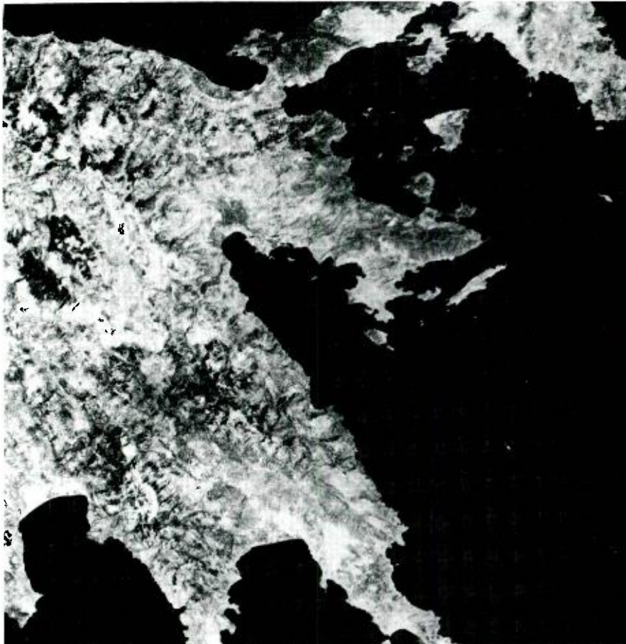
Fig. 1 — This ERTS MSS frame over Greece contains approximately 180 million bits of data. One 4-band frame is sensed and recorded every 25 seconds, telemetered to ground stations and re-recorded on high density magnetic tape. RCA 15-Mb/s digital tape recorders are employed in both spaceborne and ground station applications.
