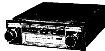
Fig. 6 — Third generation. The Model 12R703 a.m./fm/multiplex stereo radio and stereo-8 tape player for use in-dash or under-dash. This unit weighs 5.1 lbs; its dimensions are 2 1/4 in. (H) X 7 1/8 in. (W) X 7 1/8 in. (D).
