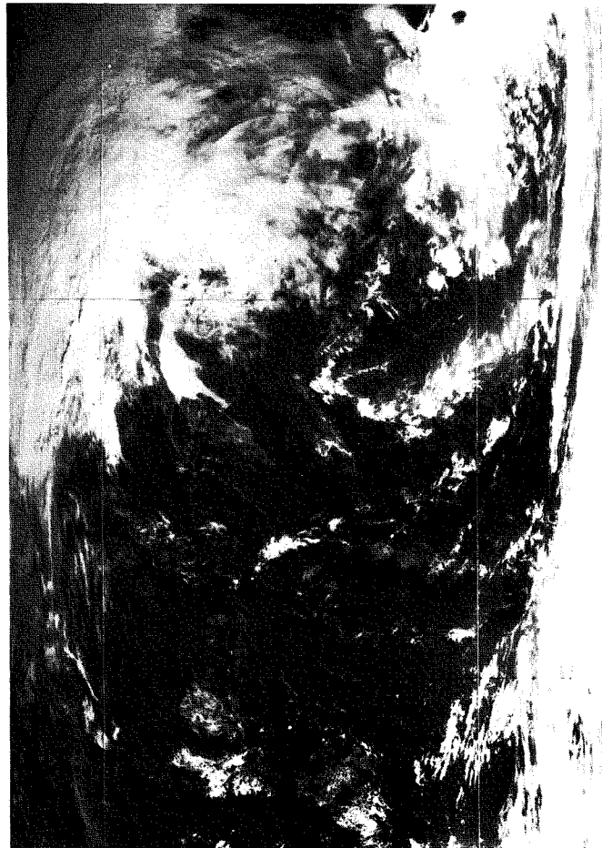
Fig. 11 — VHF simulation without geometric correction. This photo was made by performing a 4- by 3- element average over the entire image, and thus has a resulting resolution in the along-scan direction of 1.5 nmi at nadir and approximately 6.4 nmi at a local zenith of 65 degrees.
