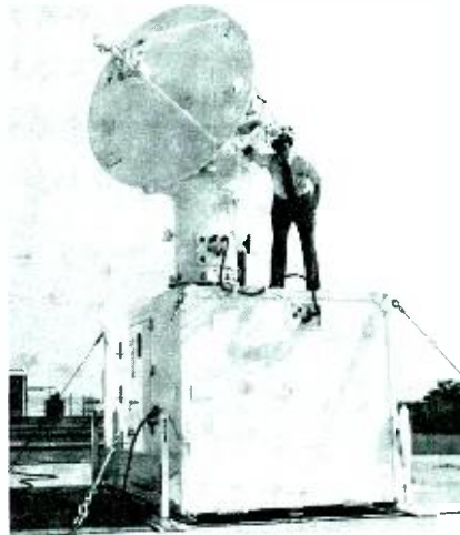
Fig. 5 — Digital Instrumentation Radar, AN/TPQ-39 is RCA's most recent range instrument, conceived and developed in 1972 as a universal range instrument.
