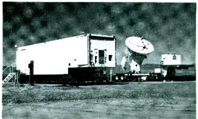
Fig. 4 — Mobile Instrumentation Radar AN/MPS-36, developed in 1970 to provide additional flexibility and mobility.
