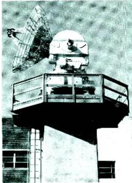
Fig. 1 — Monopulse AN/FPS-16, radarsystem developed in 1955 as a basic sensor for missile tracking.
