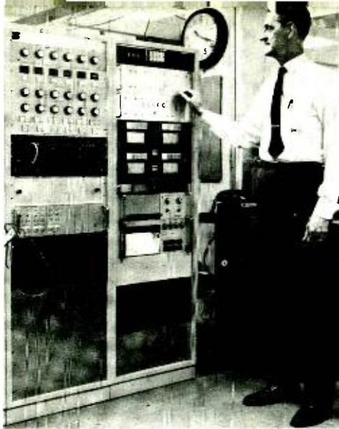
Fig. 2 — Testing six-channel level variations to drop-out recorder prototype.
