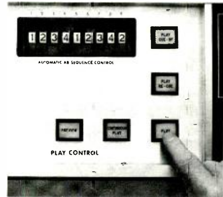
G. ... he pushes the Play button, and the program or commercial goes on air. Less than 7 seconds have elapsed since the cartridge was inserted in the bin. Note: In full automatic operation, the machine will play one cartridge after another, with no human intervention, and with no visible interruption between cartridges.
