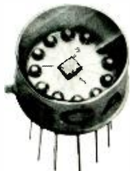
Fig. 23 (above)—Modified 12-lead TO-5 style package, CA3062. Fig. 24 (right)—Light-activated servo system. Fig. 25 (below)—Light-operated power multivibrator. Fig. 26 (below, right)—Schematic symbol of dual-gate MOS/FET with integral gate protection.
