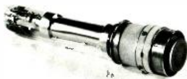
Fig. 5 — SIT sensor used in Lunar color cameras for Apollo.
