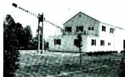
Fig. 2—This end of the antenna development facility shows the tower at one end of the radiation-pattern measurement range.
