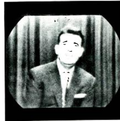
Fig. 12—Same receiver under the same conditions of excessive adjacent-channel signal as in Fig. 11, but using a synchronous detector indicating the excellent rejection of cross-modulation effects afforded by a synchronous detector.
