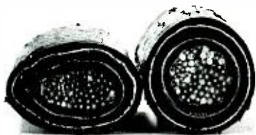
Fig. 5—Pre and Post-test condition of Minuteman cable.
