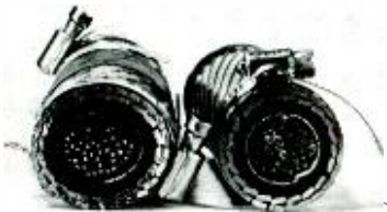
Fig. 4—Pre and Post-test condition of armored cable.
