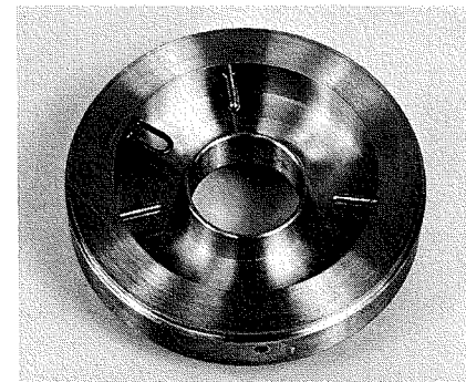
Fig. 4—A half section of the RCA 8568 klystron fourth cavity showing cavity loops and mode suppressors used to stabilize the tube.
