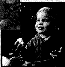
Fig. 5—Black dot 105-line "news" dot structure. Face enlargement is approximately 1.8X. Note concave-upward hum bars in actual-size reproduction; enlarged inset is shown for clarity in illustrating the "black dot" structure.
