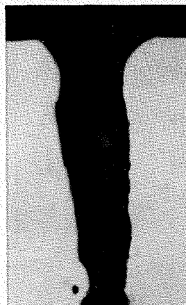
Fig. 13—Section of 0.001-inch diameter hole in 0.010-inch thick stainless steel. Non Q -switched laser.
