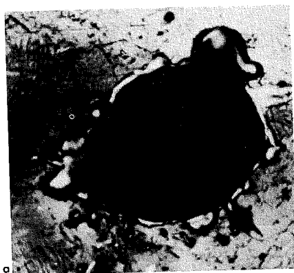
Fig. 9—Example of laser drilling in nickel. a) Hole of 0.002-inch diameter produced by non-Q-switched laser in 0.002-inch thick nickel, upper illumination. (Pulse 50% larger than used for Fig. 6b); and b) Hole of 0.002-inch diameter produced by non-Q-switched laser in 0.002-inch thick nickel, upper illumination. (Pulse 50% shorter than used for Fig. 6b).
