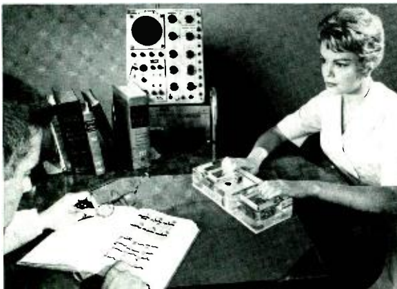
Fig. 1 — Laboratory model of an electrocardiogram transmitter. Patient dips finger into a conducting solution, and cardiogram is displayed on oscilloscope.
