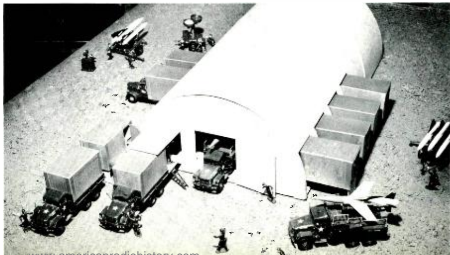
Fig. 1—An area model (40:1) used by RCA human factors engineers for synthesizing operations in an Army support system.
