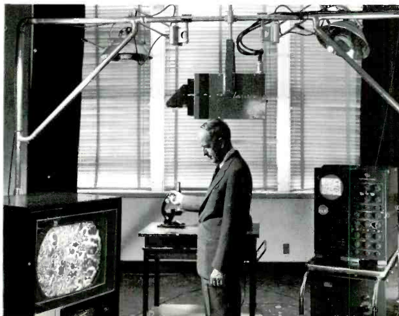
Fig. 1—The author, L. E. Flory, and a color TV system used to display images from a light microscope.
