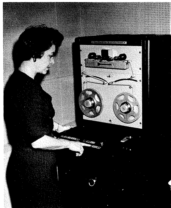
Fig. 2—RCA Datatelex used at Socony Mobil for overseas transmission; input data such as magnetic tape, paper tape, and punched-card forms can be sent by Datatelex.
