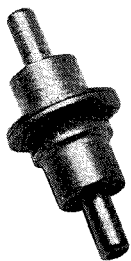
Fig. 1—RCA high power epitaxial silicon varactor diode (Dev. No. VD500 series).
