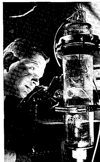
Fig. 4—G. A. Swartz examining experimental RF plasma propulsion experiment.
