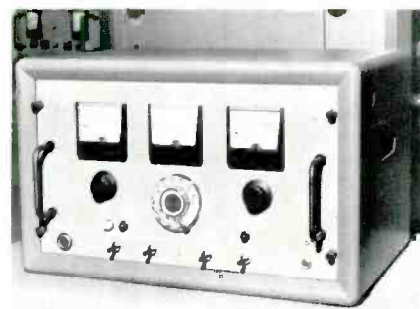
Fig. 3—The companion remote control unit is designed to fit on a desk-top, or may be mounted in a standard 19" cabinet rack. The remote unit provides master "telephone-dial" control of the IST-5K transmitter's automatic circuits over distances up to 10 miles.
