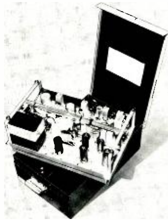
Fig. 2—E-Line 450-Mc transmitter-receiver.
