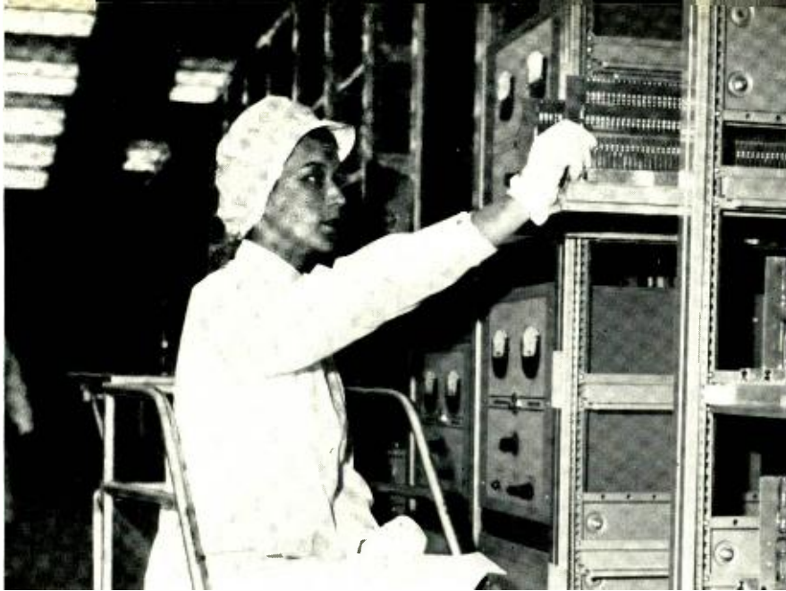
Fig. 2—White Room worker inserting component matrix boards in pre-conditioning racks
