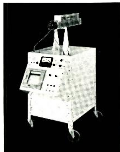
Fig. 4—Ion density measuring equipment.
