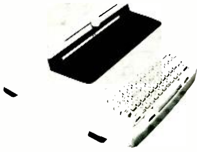
Fig. 6—Engineering model of the electroluminescent verifying keyboard.
