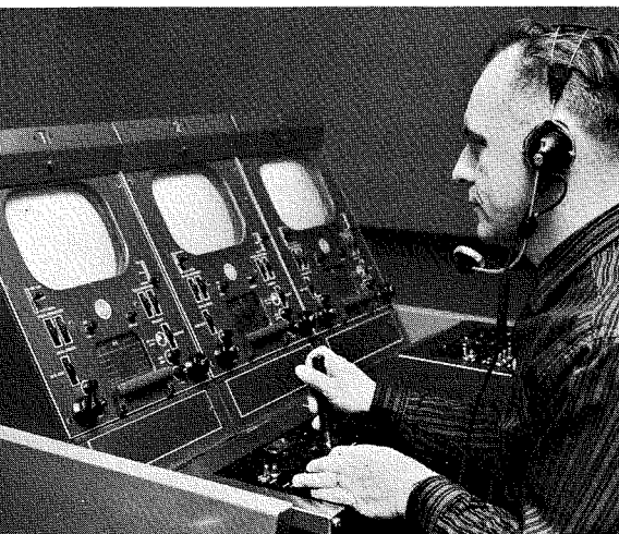
Fig. 1—Remote control of robot TV cameras. Operator is using "joy stick" for pan and tilt; with his left hand he operates switches for zoom and focus.
