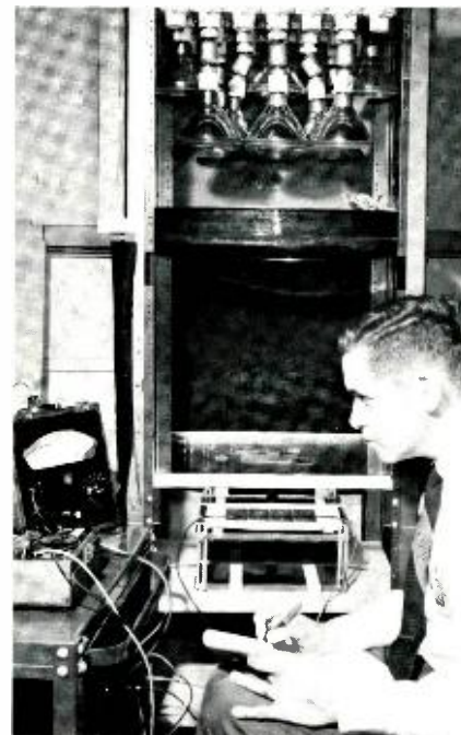
Fig. 1—P. Wiener works with solar-illumination simulator being used here to test electrical output of a module of 80 solar cells.
