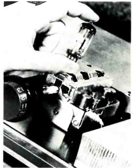
Fig. 6—Experimental "Nuvistorized" tuner capable of superior performance with plate voltage of 40 volts. Conventional tube used in present-day TV tuners is held in hand for comparison with thimble-size Nuvistor.
