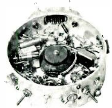
Fig. 3—Typical satellite beacon transmitter; weight 0.5 pound.
