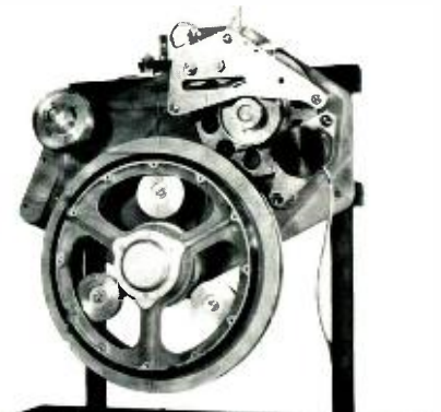
Fig. 4—Magnetic-tape transport for video storage on board a satellite. Tape speed is 50 ips, with a 1½-minute running time.
