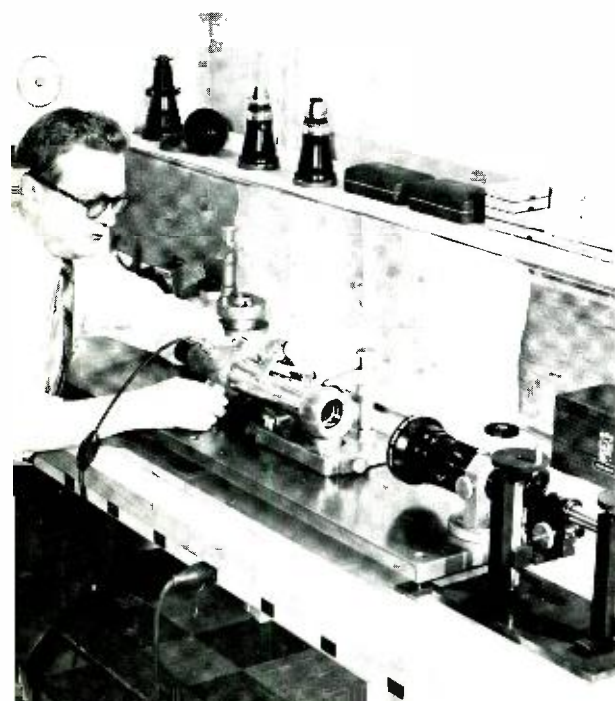
Fig. 6—R. Jordan determines focus properties of lenses for satellite TV-cameras in a dust-free area.
