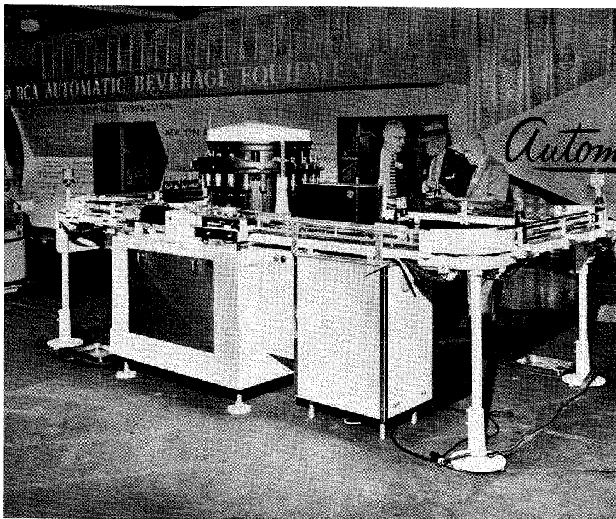
View of complete beverage inspection machine as displayed at a recent National Convention.
