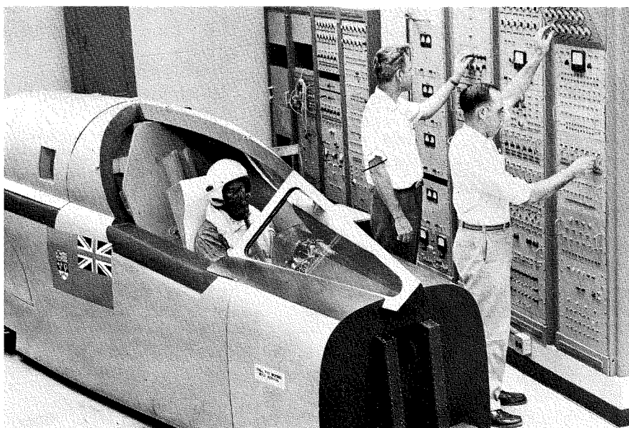
Cockpit simulators have been built by RCA to permit the analysis of complicated fire control systems problems in which a human operator performs a part of the mission. Left to right are technicians R. J. Geehan (in cockpit), Kevin Ronan, and Courtland Baird.
