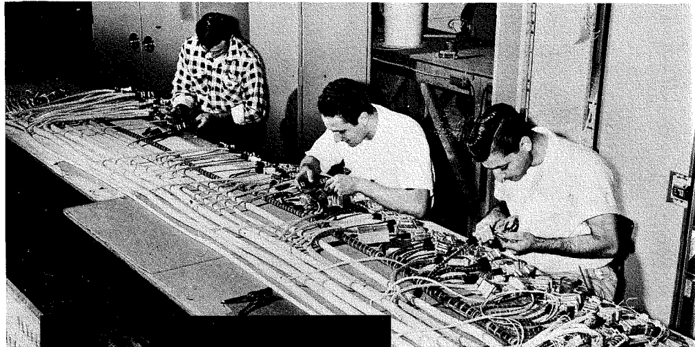
Fig. 3—An example of the intricate cable-lacing techniques in use in Moorestown. (L to R) Messrs. DeChurches, Pantaloni and Martinelli are shown inserting pins in plugs on an overhead harness.
