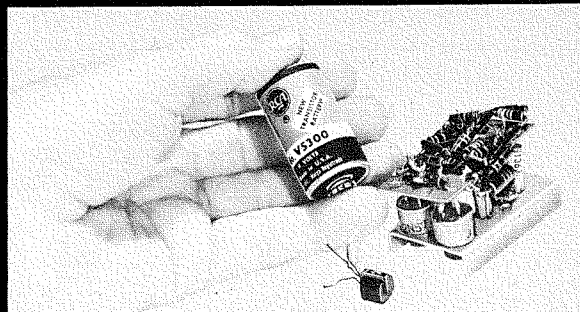
Fig. 2—Transistorized servo-amplifiers are adaptable for use with printed circuits. (L to R) H. W. Day, W. R. Bauer, J. V. Landis, Mgr., Inductive Components and J. C. Koenigsberg discuss methods of applying printed circuit techniques to transistorized amplifiers. Compare the size of the Servo Amplifier (held by Mr. Day and also shown in hand with miniature battery) to the size of a common output transformer held by Mr. Landis. Note that transistorized servo amplifier is about same size as transistor battery. Miniature input transformer is removed so readers can see relative size.
