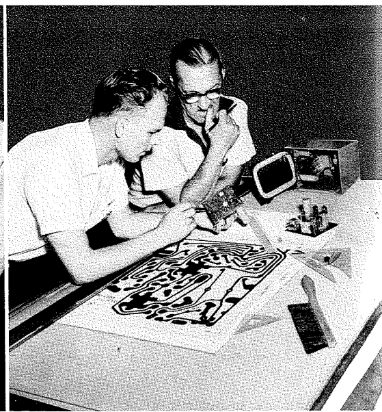
Fig. 11—Robert D. Short (l), mechanical engineer and J. K. Forman, draftsman of the Radio and "Victrola" Division, checking a printed wiring circuit board for clearance between wiring points. On the table is the photomaster.
