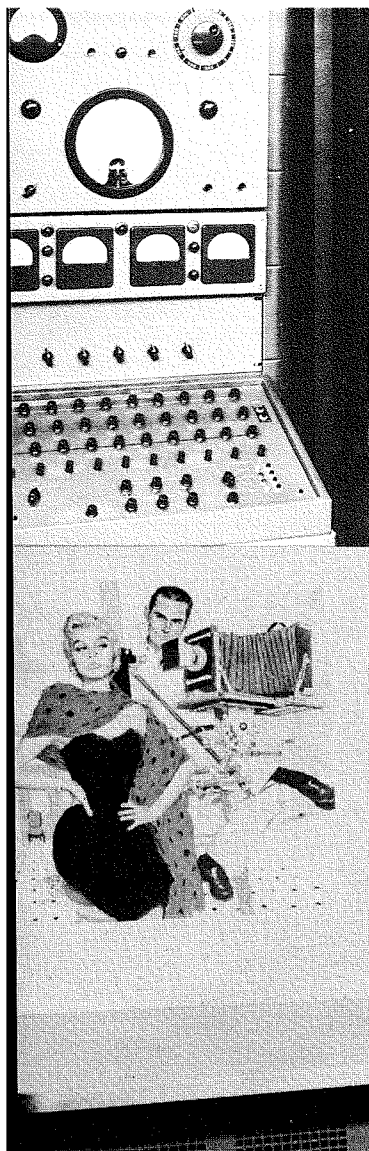
Fig. 2—Electronic Control Panel—The symmetrical array of 27 knobs represents the 9 x 3 Neugebauer matrix for adjustment of computer constants. Other controls are for the purpose of adjusting scanning and recording light levels and generally operating the equipment.
