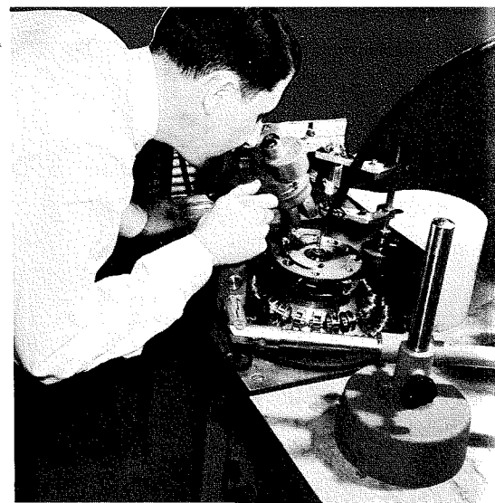
Fig. 4—H. J. Ackerman, Tube Division Mechanical Engineer, checks alignment of wires in Vertical Grid for Pencil Tubes. Machine automatically draws vertical wires from spools at bottom, winds a helix coil around them, and R-F brazes each cross-over point.
