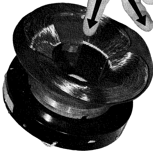
Fig. 1—Relationship between direction of beam current (forefinger), which is opposite to that of electron travel, horizontal-coil flux (middle finger), and resulting deflecting force (thumb) as illustrated by the "right-hand screw" rule.
