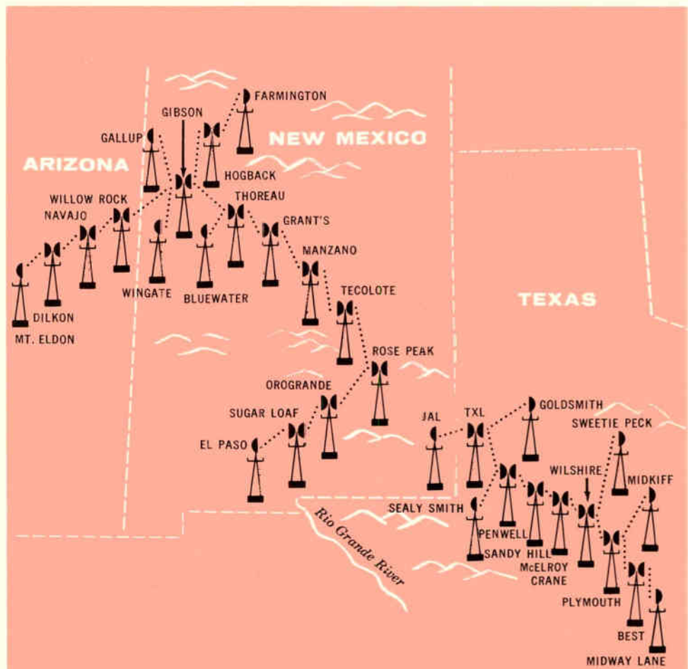
Fig. 9—Map shows present location of microwave installations on El Paso's ever-expanding communications system.
