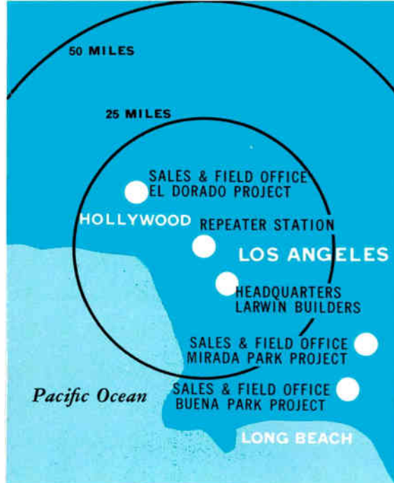
Fig. 3—Map shows location of Larwin headquarters and three building projects. Repeater station in Hollywood Hills boosts radio signal to cover 50 mile area.
