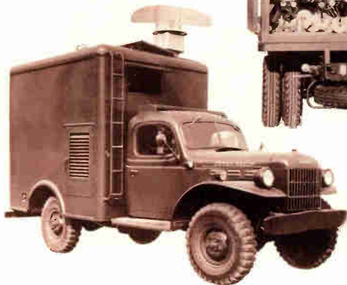
Fig. 5—Radar Truck—One of mobile units which supplement the fixed Microwave system.
