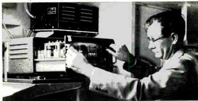
Fig. 4—As an aid to navigation, Loran is constantly relied upon by skippers. Technician E. E. McCarthy removes chassis of unit aboard SS UNITED STATES prior to inspection.
