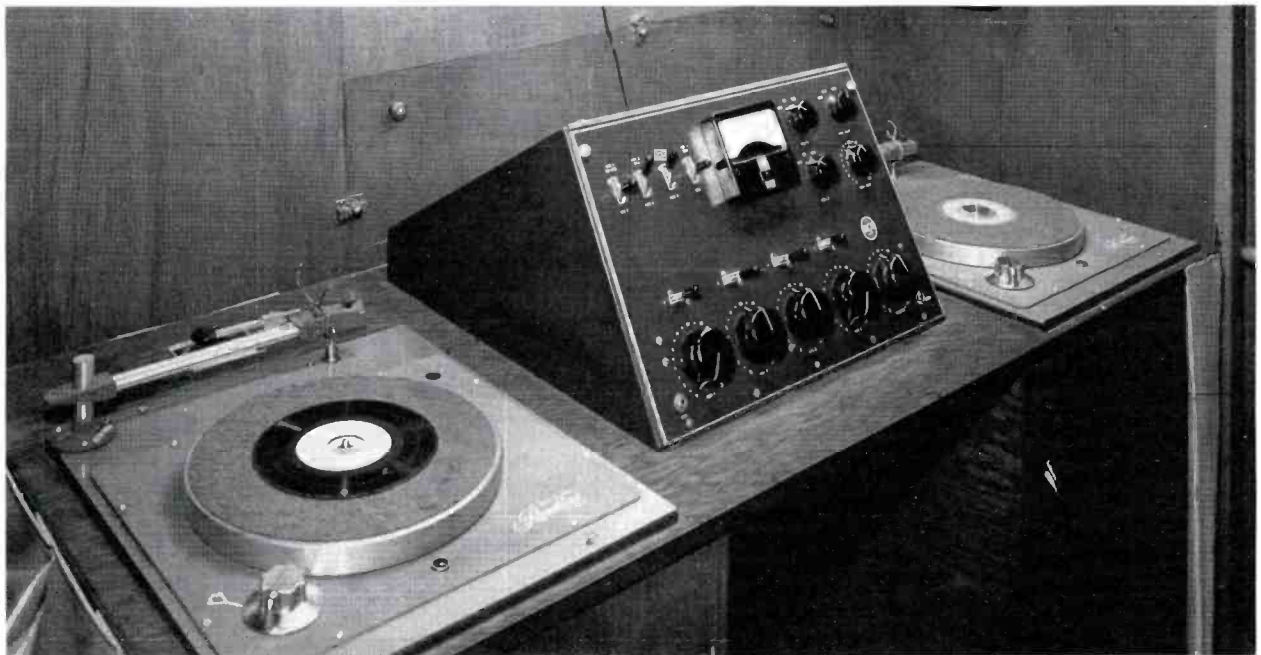
FIG. 6. Control console inside WERE mobile unit. Three-speed turntables are used. An RCA Type BC-5A Audio-Console is employed. The complete control console can be removed as a unit for use in semipermanent remotes.
