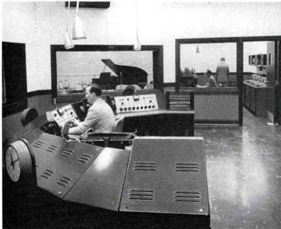
FIG. 47. Another view of WBT radio control room, showing direct access to recording room (top right). Recording equipment can be operated independently or by push-button control from master.
