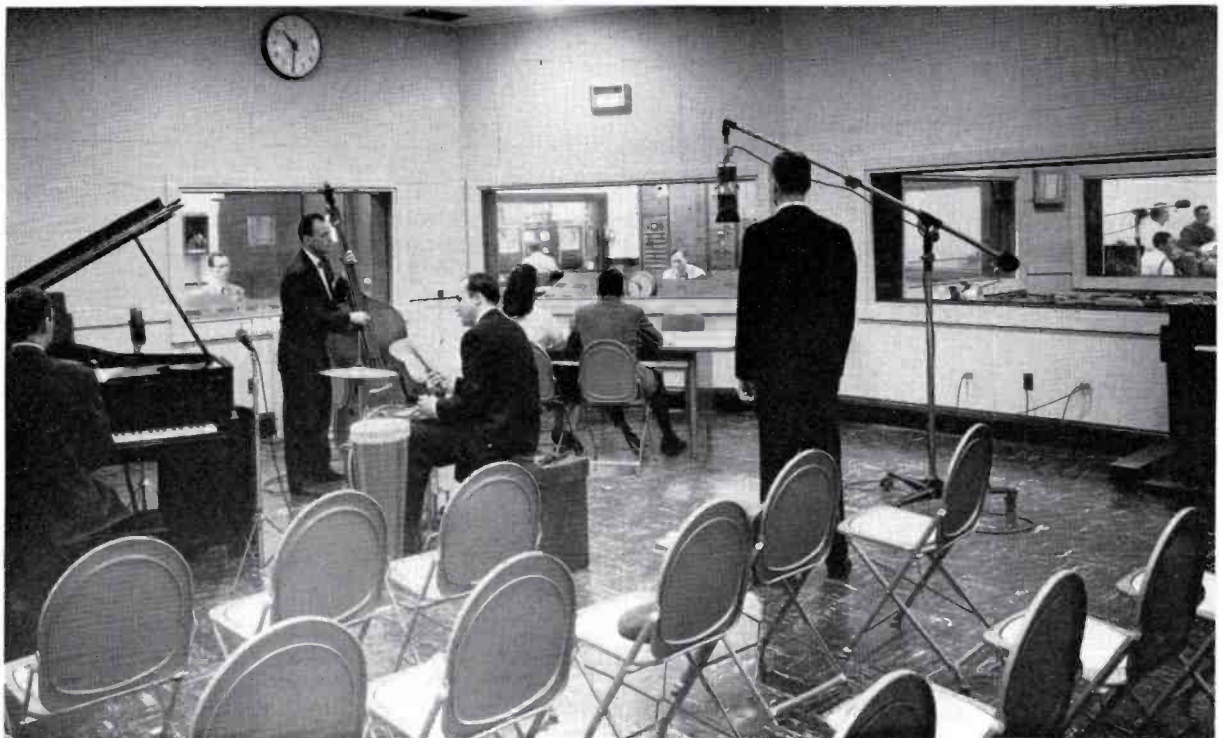
FIG. 46. Not only are the technical operations of WBT-WBTV centered in one area but, for convenience, the whole area is made visible by conveniently placed windows. In this view, from Studio C, can be seen the recording room (left); the radio control room, and beyond it the tv control room (center); and Studios B and A (right).
