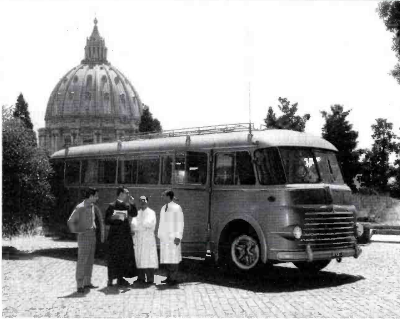
FIG. 29. One of two RCA-equipped mobile units used by Vatican Radio for remotes from basilicas, churches and special events within a 35-mile radius of St. Peter's.
