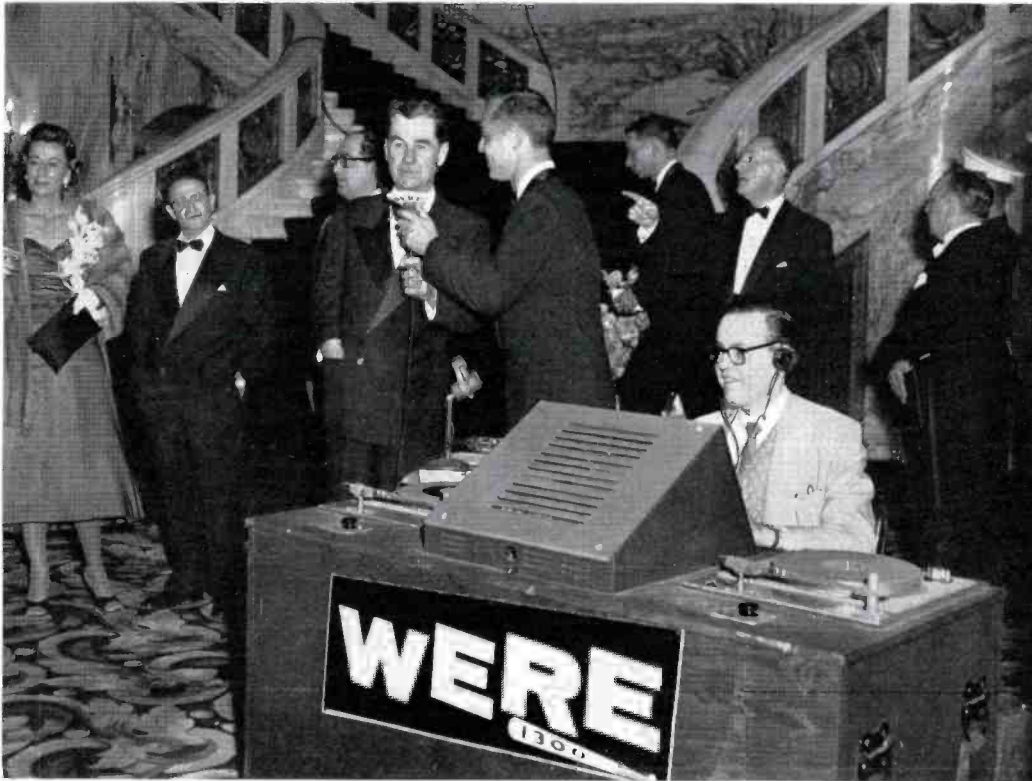
FIG. 3. Single-package remote unit designed by WERE Engineering Staff. It weighs only 70 lb., including two turntables, amplifiers, PA system and audio-console. Note handles for carrying. This is easily moved from one location to another.
