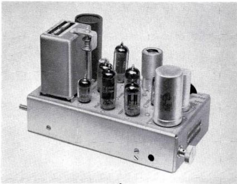
FIG. 10. Video amplifier in the processing amplifier contains a plug-in gamma compensation unit (front left). Unit has gradient correction of 0.7 which can be switched in-or-out at the control panel.
