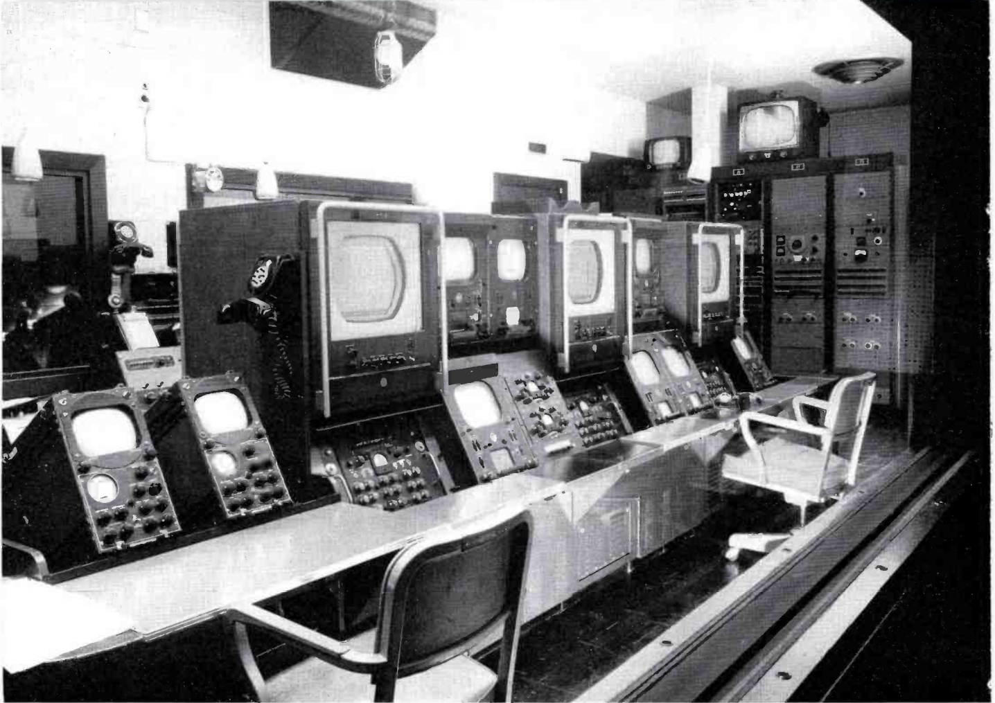
FIG. 18. WBTB's video control console as seen through the window from the a-m control room (see floor plan, Fig. 6). Camera control for four monochrome studio cameras, one color studio camera, two 3-V color film cameras and two color Chromascan units are incorporated in this console. Monitors are provided for both monochrome and color operation. Location of the various units in this console is shown in Fig. 19. Video operators at this position make all necessary camera adjustments. Camera switching is done by the director in the studio control booth.
