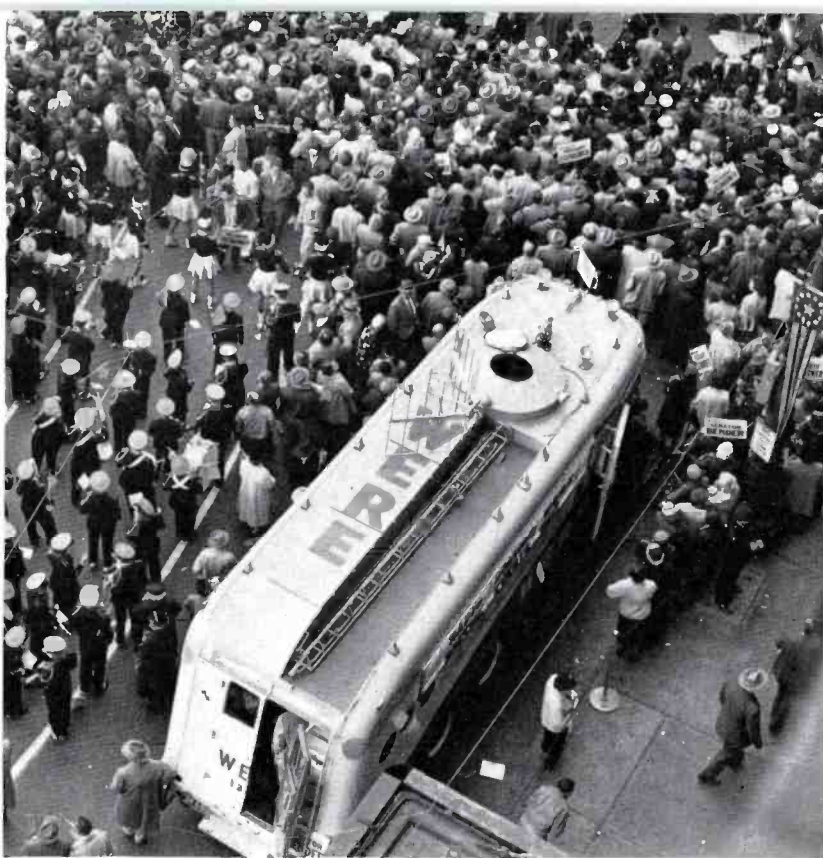
FIG. 4A. WERE mobile unit in use at the 1956 presidential political campaign meetings. Note that turret is in "recessed" position.
