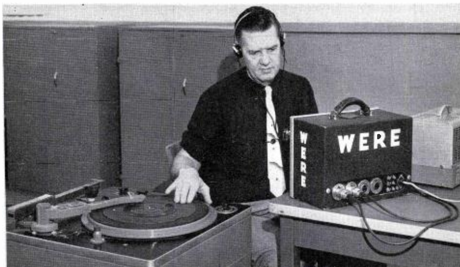
FIG. 1. Equipment once used for remote disc-jockey type pick ups. This included heavy, studio-type 70-D turntable, remote amplifier and other necessary equipment. It was a bulky lot, very inconvenient to move from place to place.
