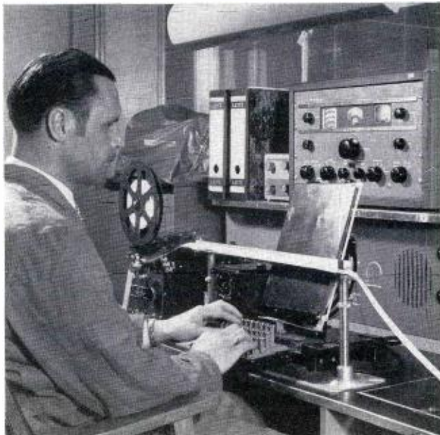
FIG. 20. Monitoring is by four methods: Direct-Voice, radio teletype, Hellschreiber, and Morse code. Here is an operator receiving Morse code and transcribing it on a teletype perforating machine.
