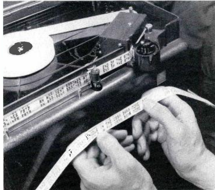
FIG. 21. Typical output of a Hellschreiber recorder. This is being fed from an RCA Communications receiver. The monitoring output at Schleissheim is fed to Munich via telephone lines.
