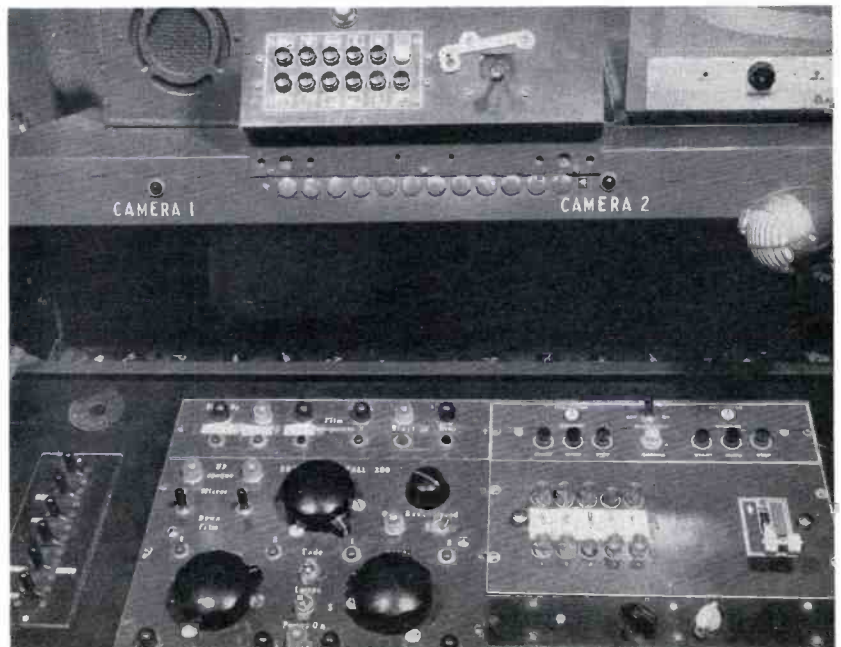
FIG. 15. Closeup of WISH-TV subcontrol console showing Technical Director's position. At top is control panel for video effects equipment. Keys at left for plant intercom. Center panels for remote control of monochrome projector No. 3, slides, and opaques. Right hand panels from top to bottom: projector controls for color projectors, TS-5 switcher, and switching panel (black and white knobs) for connecting video into effects equipment.
