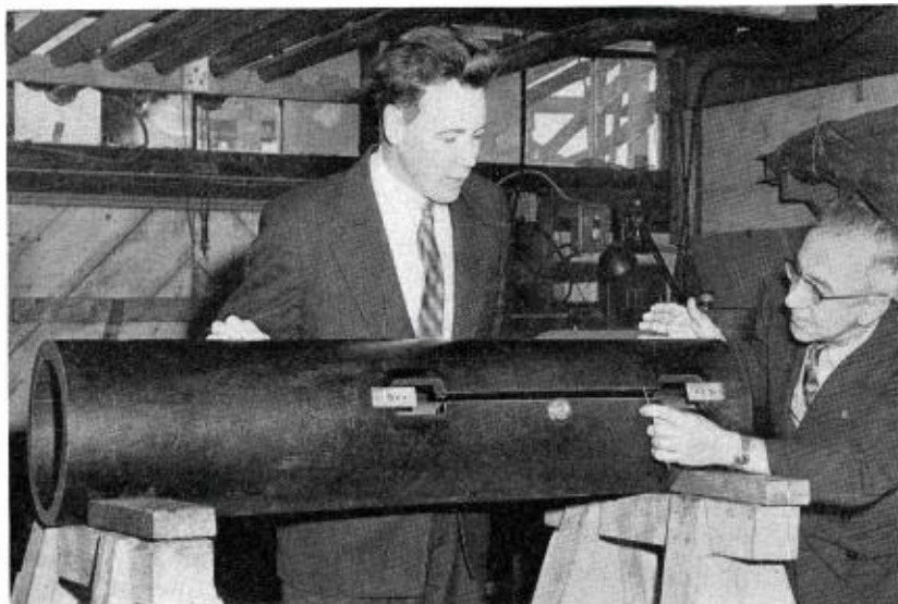
FIG. 7. Final inductively tuned slots for a gain of 9 antenna on 10 3/4 inch diameter pole section being inspected by the authors, Matti S. Stukola (left) and George A. Kumpf.
