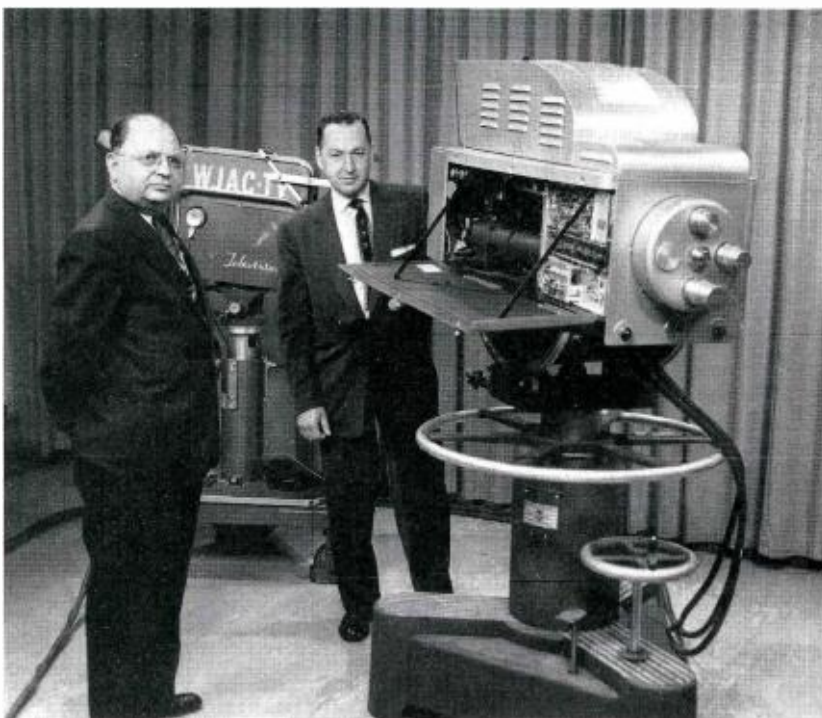
Nevin L. Straub, WJAC Director of Technical Operations (left) and R. S. (Bob) Emch, RCA Cleveland Office, examining new RCA TK-41 Live Color Camera Chain.
