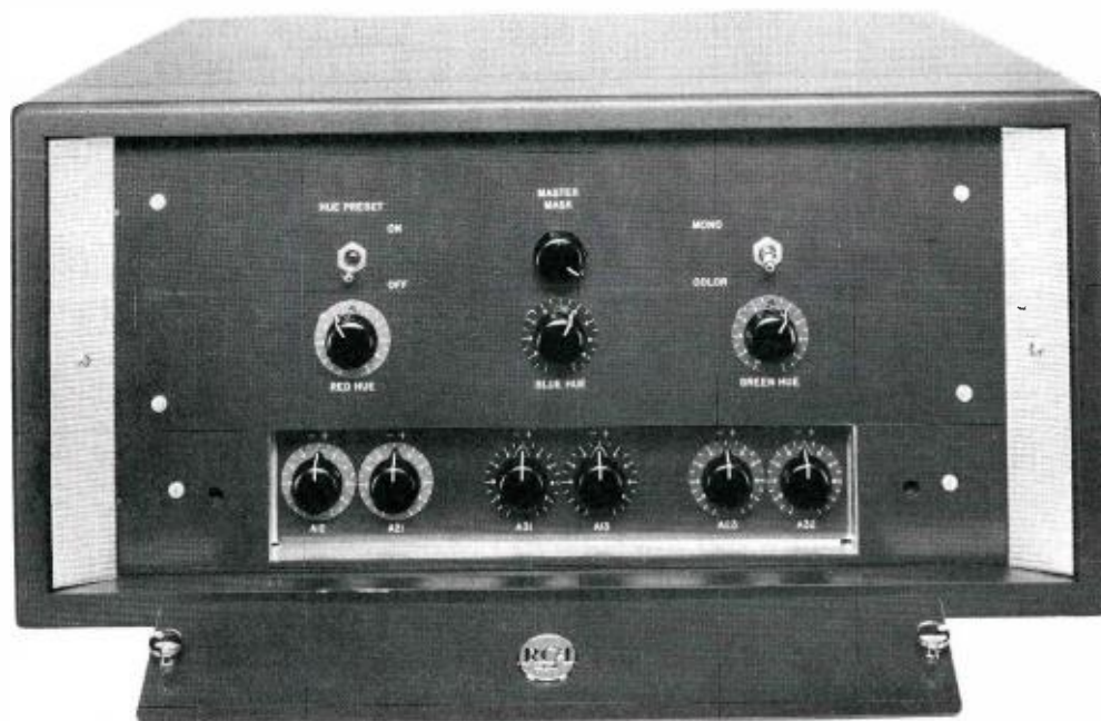
FIG. 1. Masking amplifier with front plate removed to show the six independent coefficient control knobs.
