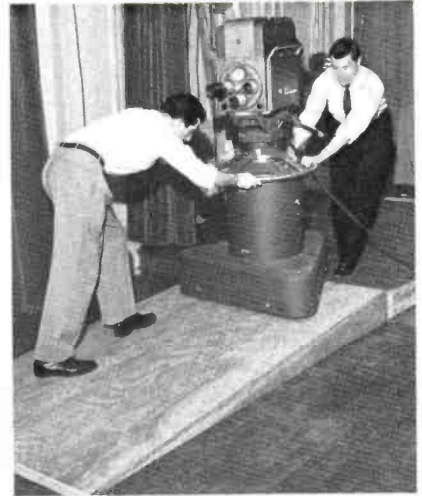
FIG. 25. A special ramp was constructed so that cameras might easily be rolled on or off the platform as might be required.
