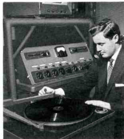
FIG 28. RCA audio console handles inputs from the turntable shown plus studio microphones and tape recorders.
