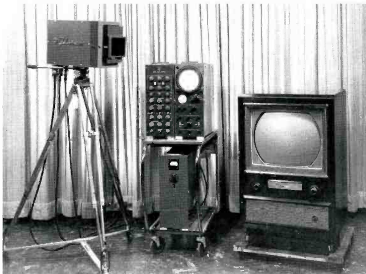
FIG. 3. A color camera chain developed at Princeton was used in some of the demonstrations. Equipments shown include: the color camera, camera control unit, camera control monitor, power supply and color receiver.
