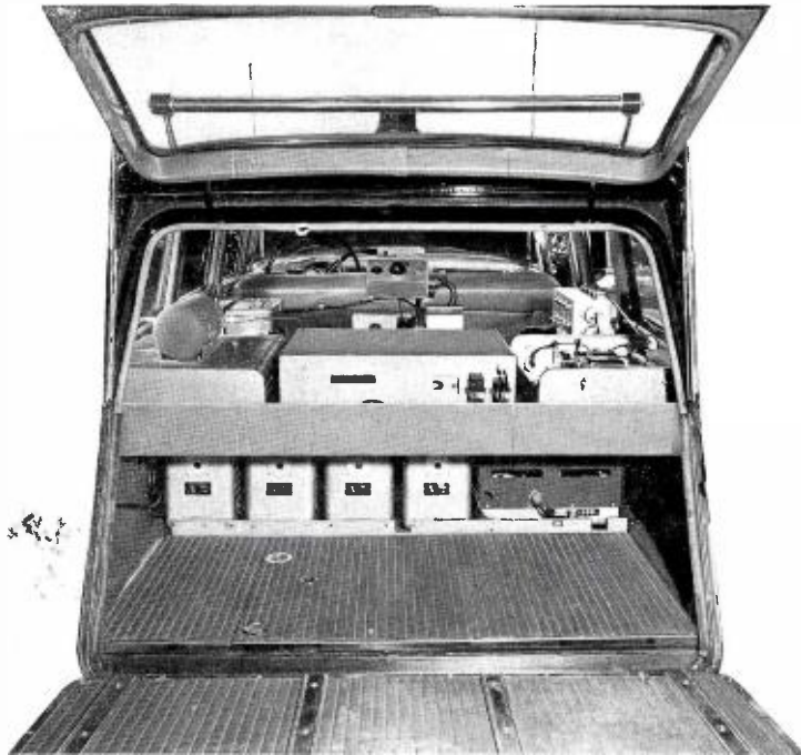
FIG. 4. Rear view of station wagon showing rear of ATR units with view of the control unit mounted on back of front seat so that driver may operate the equipment. Note that floor plate is free for removal to get at spare tire.
