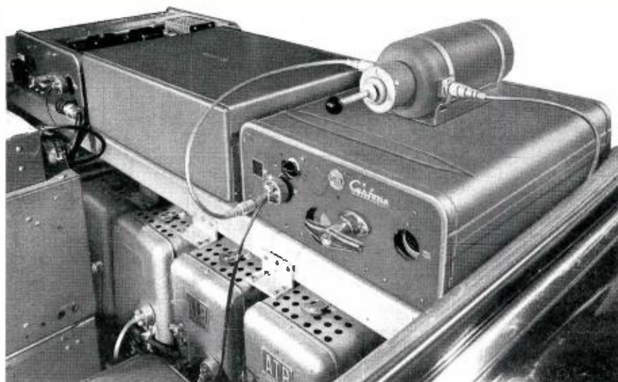
FIG. 6. Close-up of (left-to-right) RCA CARFONE Transmitter, Bell Telephone Receiver, RCA CARFONE Receiver.
