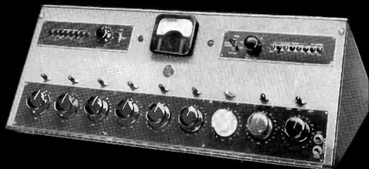
BC-2B STUDIO CONSOLE. "Low-boy" console offers deluxe, operation-proved features usually found in custom-built equipment—but at a standard "package" price. Includes complete high-fidelity speech input provisions for 2 studios, announce booth, 2 turntables, 5 remotes, and network.
