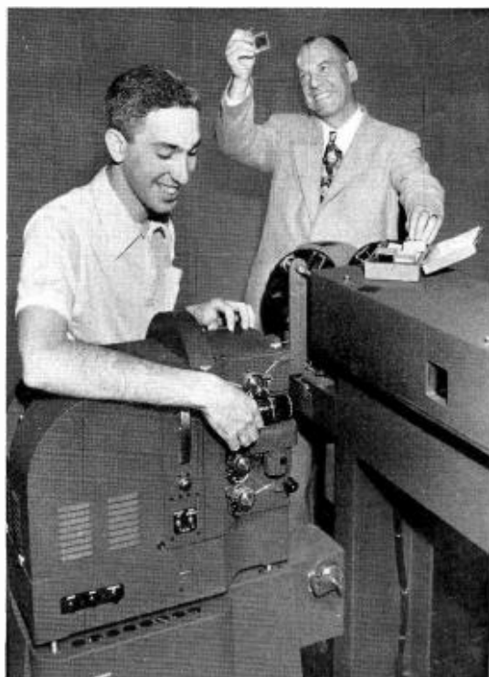
Vidicon film facilities at WQED. Two RCA TP-16 16mm film projectors and a dual disc slide projector are used with the RCA TP-11 vidicon multiplexer and TK-21 vidicon film camera.
