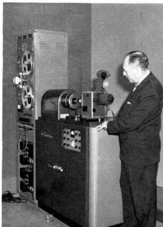
RCA TMP-20B kinephoto recording equipment. Kinescope films of WQED's most successful programs are produced here for national distribution through the Ford Foundation film center.
