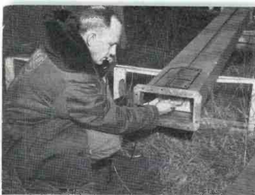
FIG. 2. F. J. McMenamin adjusts temporary shorting plate at end of a test length of waveguide (shown below, Fig. 3) for product development test.
