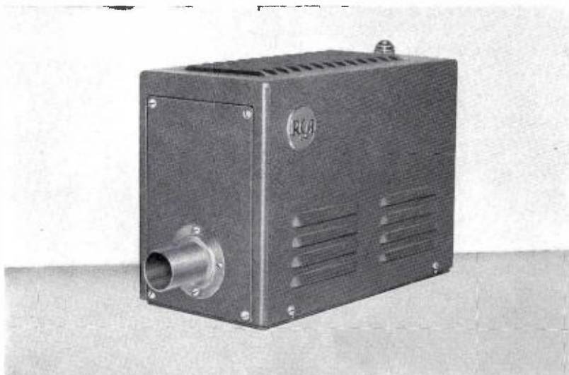
FIG. 3. Overall view of the Vidicon Camera unit when removed from projector setup.
