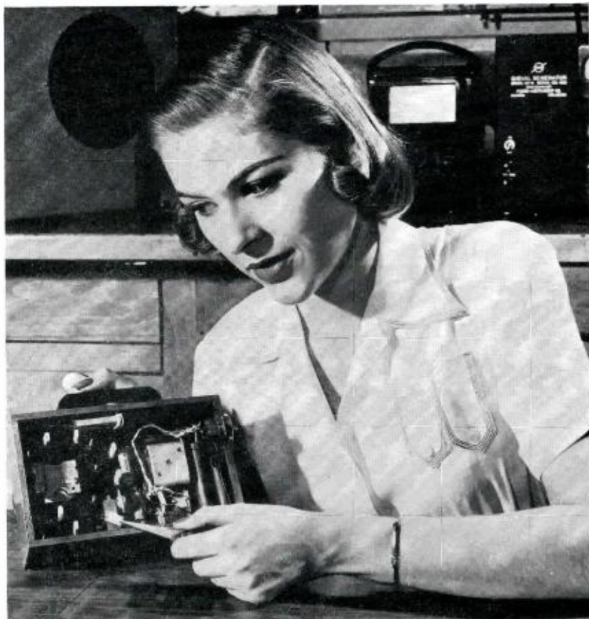
FIG. 17. Transistors in an experimental personal-type AM receiver developed at the David Sarnoff Research Center of RCA at Princeton, N. J., permit tremendous reduction in size, battery weight and power consumption.
