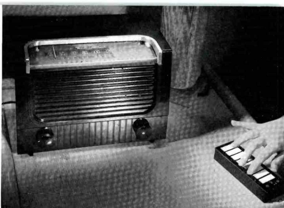
FIG. 8. Toy "piano" operated by one transistor and small battery. This experimental electronic keyboard contains one developmental junction type transistor and eight frequency-selecting circuits—one for each key. Complete scale is produced when "transmitting" to standard broadcast receiver.
