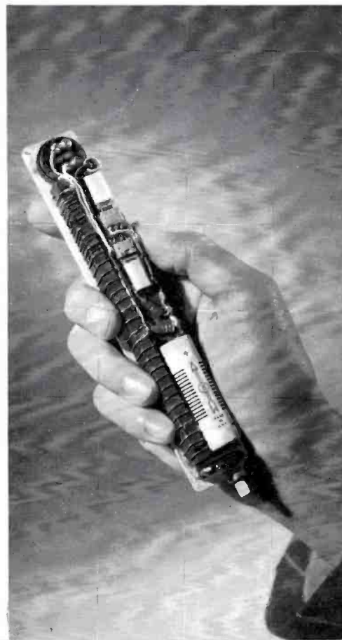
FIG. 7. A cigar-size experimental microphone-transmitter, modulated by a tiny built-in dynamic microphone. Employs two developmental junction type transistors, coil and battery.
