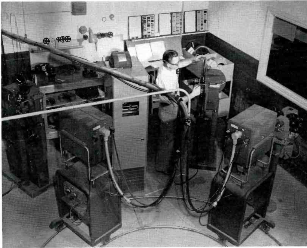
FIG. 2. The film projection room at KBTV allows for complete simplicity of operation. Two film projectors and slide projector are conveniently located for speed.
