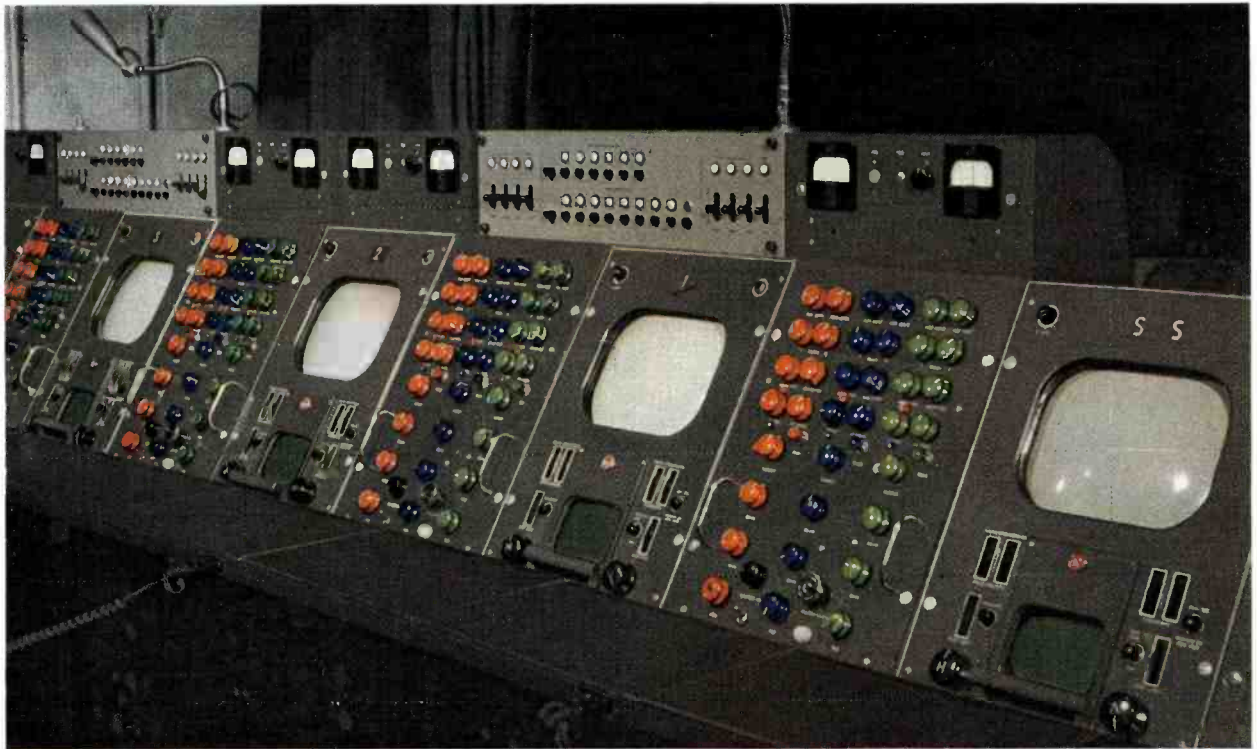
FIG. 1. Camera Control Console in the control room of NBC's Colonial Theatre Color Studio. Four RCA Color Cameras are controlled from this position. Each camera "chain" includes a camera control unit (the panels with a large number of knobs) and a modified Type TM-5B master monitor (used for monochrome monitoring).
