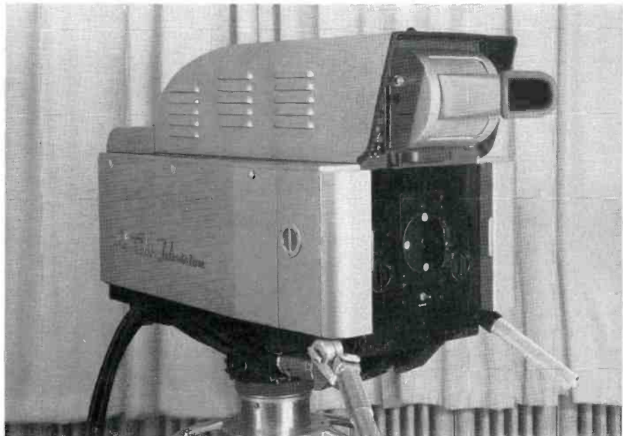
FIG. 6. Rear view of RCA Color Camera with viewing hood in place.
