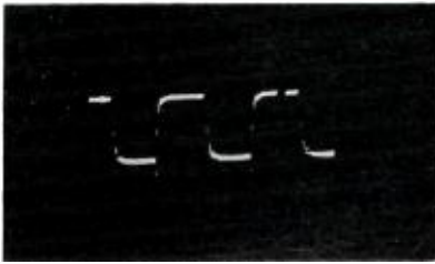
FIG. 22. Square wave out of transmitter and demodulator before and after delay equalization.
