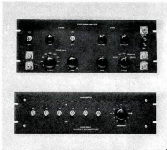
FIG. 4. The Color Signal Analyzer is used for measuring phase of subcarrier frequency. Along with Linearity Checker it is used for phase intermodulation checks.
