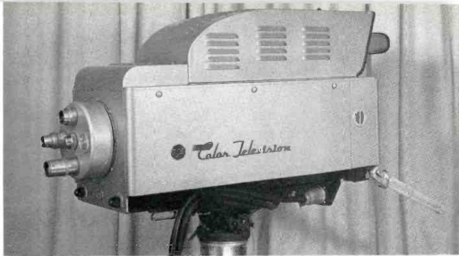
FIG. 5. Side view of "all electronic" RCA Color Camera and Viewfinder.
