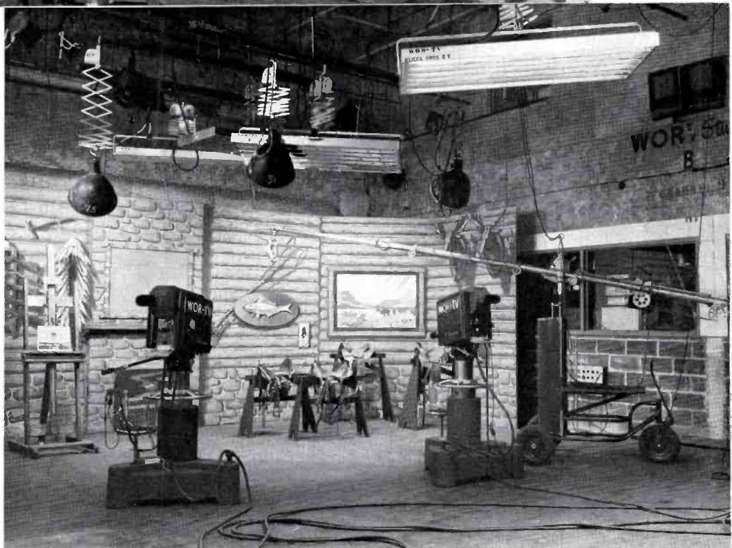
FIG. 7. View of studio "B" setup, as made ready for the "B.B.A.R.B." Program. Four cameras are available for use in each of the large studios which provide an unusually flexible playing area.
