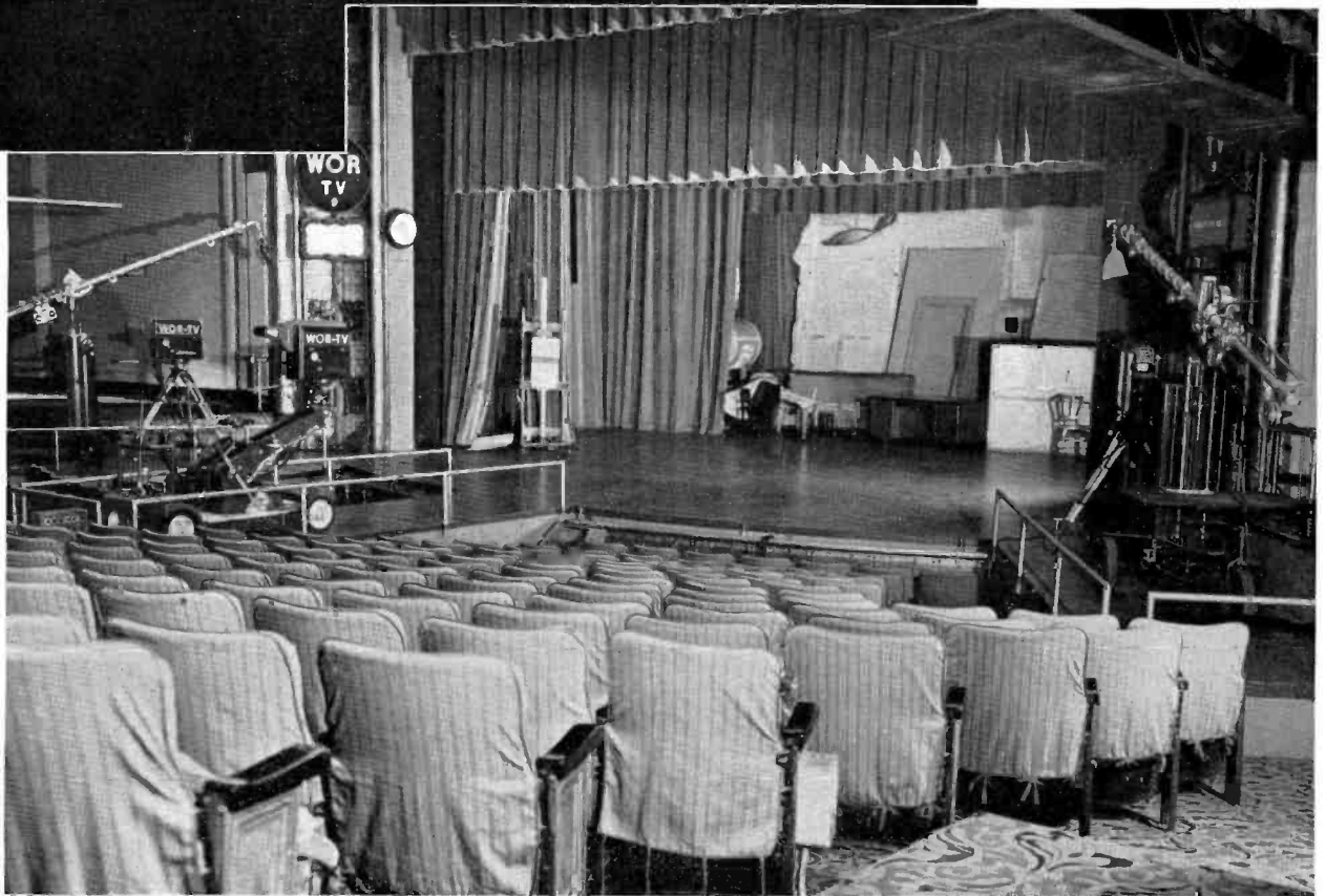
FIG. 41. Overall view of the New Amsterdam Theatre studio showing the studio facilities available. Three television cameras and two mike booms are visible on the respective ramps. At center ramp, a studio camera is mounted on a two-man dolly. ▼
