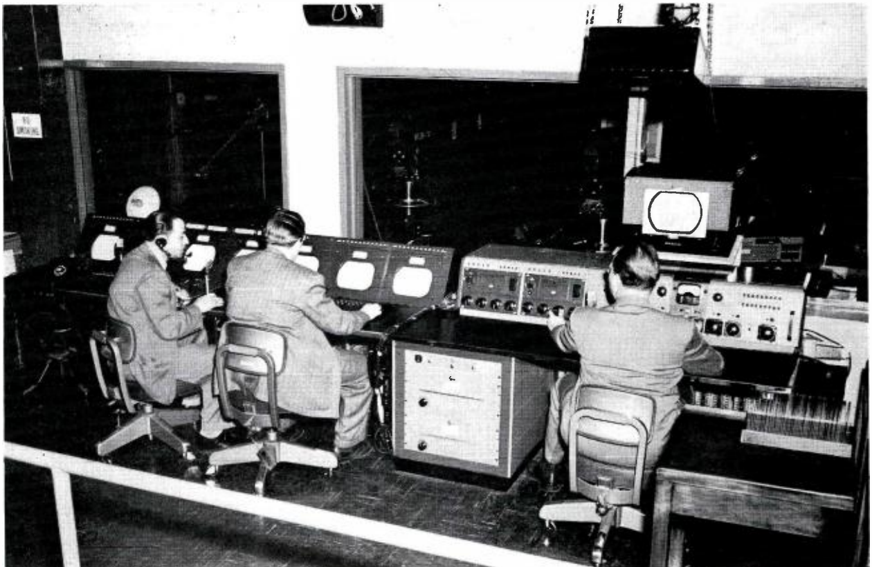
FIG. 12 (below). Studio Control Room "B" during program operation (Program Director at left watches seven monitors; Preview 1, Cameras 1, 2, 3 and 4, Preview 2 and Line Monitor). Video Switcher sits at director's right and audio engineer at audio mixing controls.
