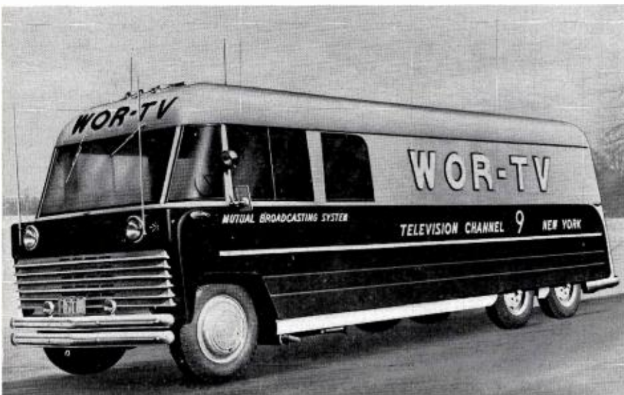
FIG. 44. "Johnny-on-the-Spot." WOR-TV's Mobile Unit is equipped with three field cameras, microwave transmitter, camera control units, video picture monitors, and camera switching equipment. In addition, the unit houses a radio telephone and AM broadcasting equipment.
