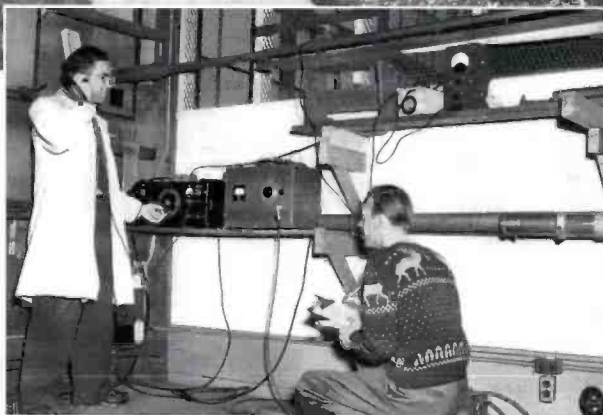
FIG. 5. Richard Wright and Joseph Blake are shown making characteristic impedance measurements on the Super Turnstile Antenna pictured in Fig. 4.
