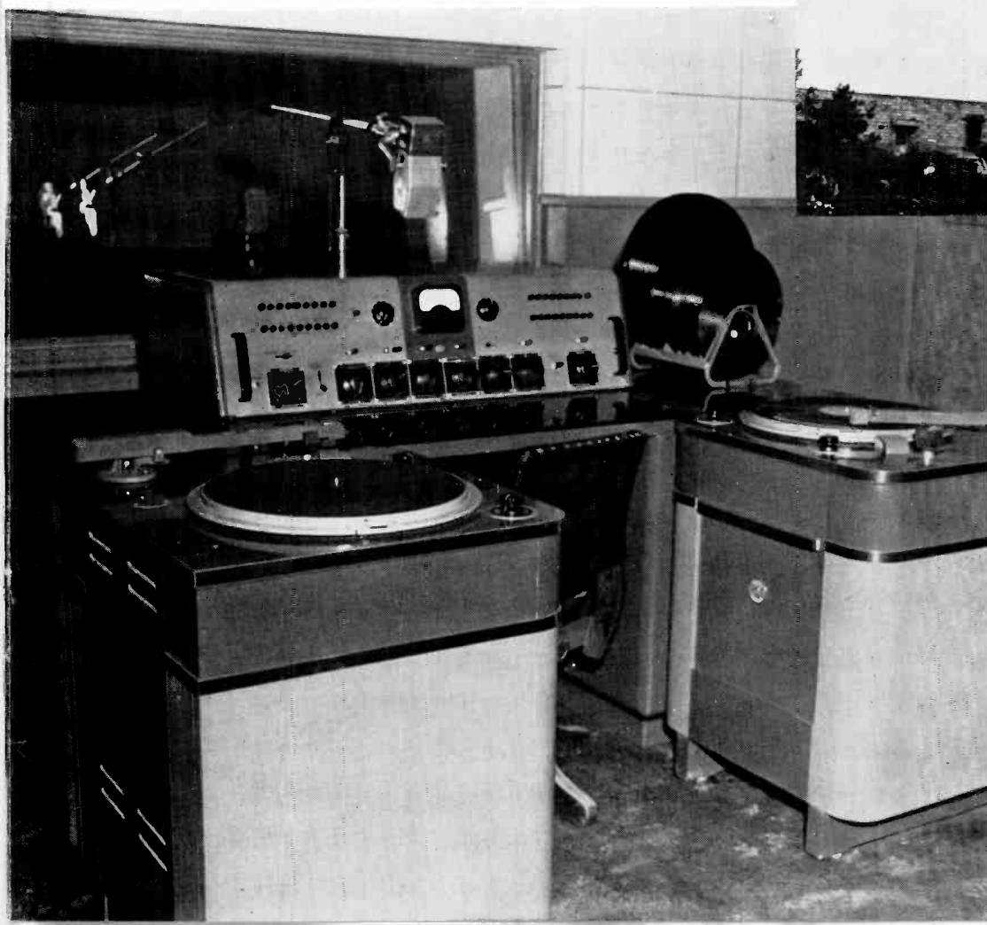
Left: Studio control room of WBRE-FM, like the rest of the station, is 100% RCA-equipped. The standard 76-B console is flanked by a 70-C-2 turntable. Through the window may be seen the studio with its 44-BX microphones.
