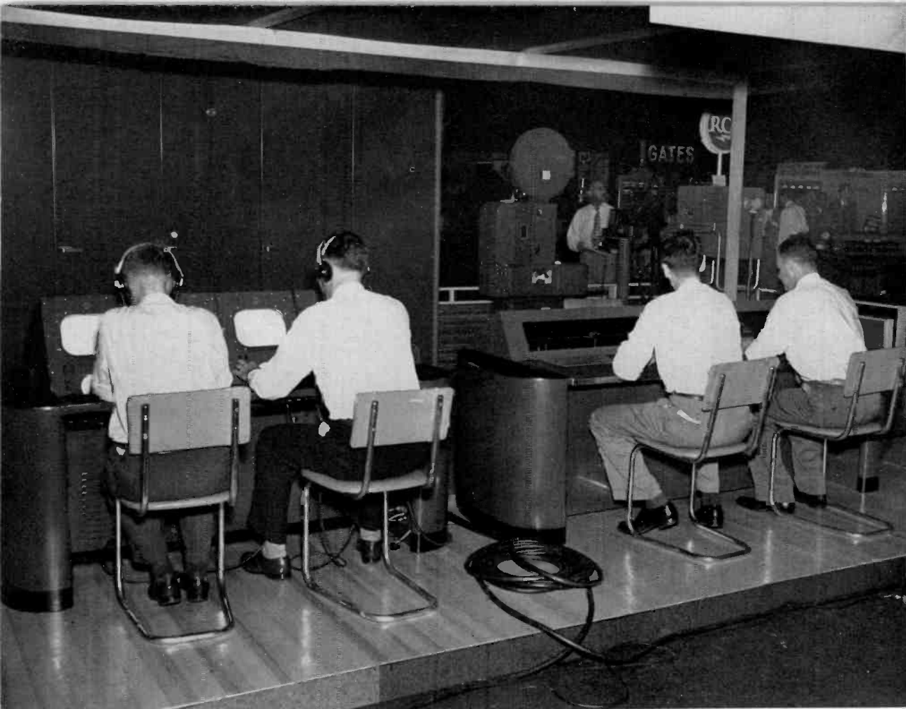
(Above) This closeup view shows the video control and program director's consoles in actual operation, as they were during hours the exhibits were open. Seated at the controls, from left to right, are John Roe, L. E. Anderson, W. J. Poch and George Jacobs of the RCA Television Terminal Equipment Engineering Section.
