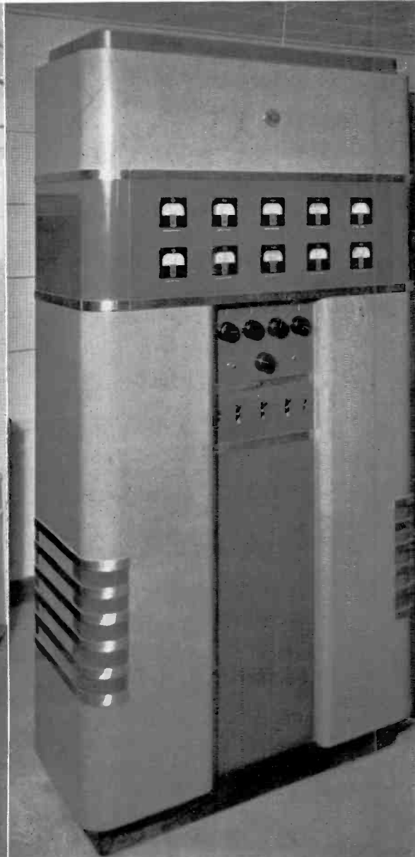
FIG. 2. (below) Llewellyn Jones, Chief Engineer, at the controls of the WSBA 1-kilowatt AM transmitter, RCA Type 1-K.
