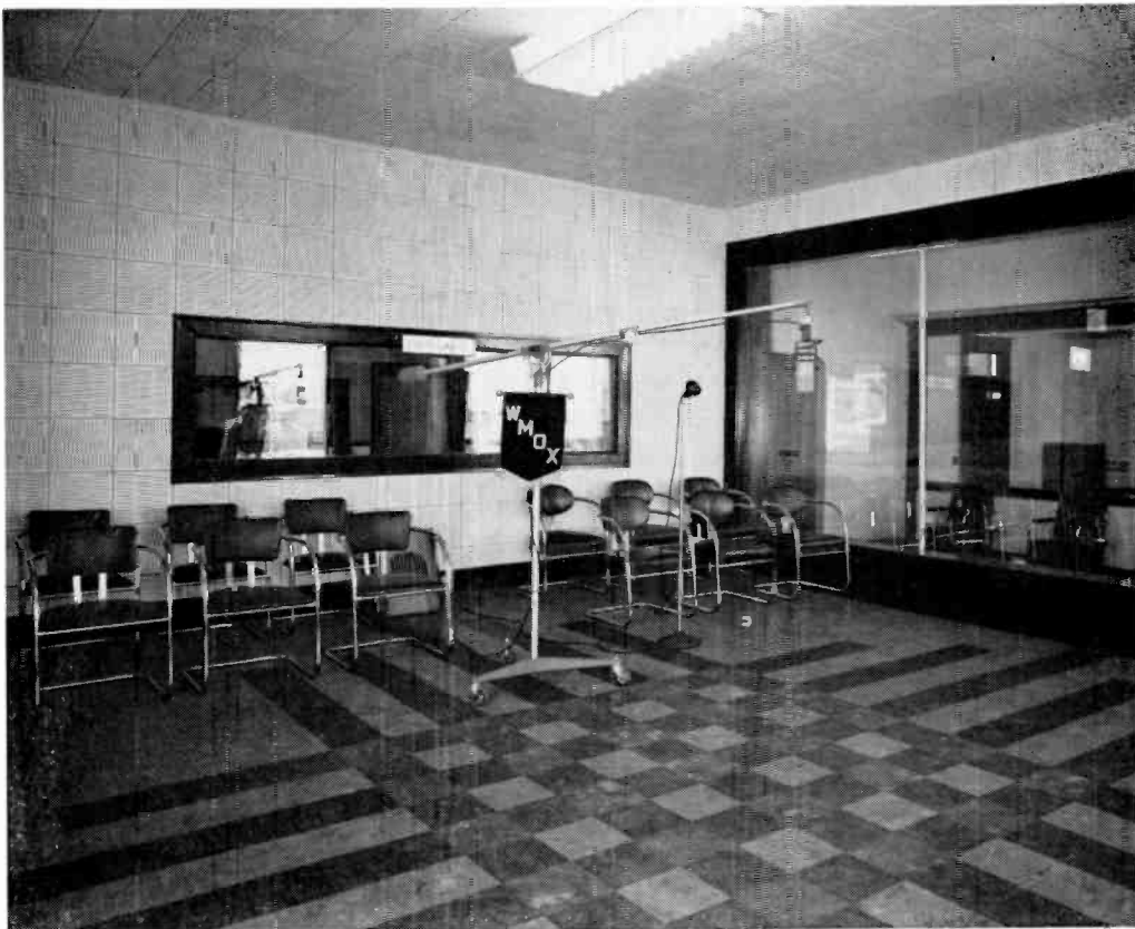
FIG. 2. (Right) A corner of WMOX's Studio A, looking toward the control room. Lobby and offices are to the right. Microphones include an 88-A and 44-BX on a boom stand. WMOX's Studio B, which is not shown, is 25 feet by 30 feet in size and has a skylight which provides an interesting daylight effect. Type 44-BX's are also used in this studio.
