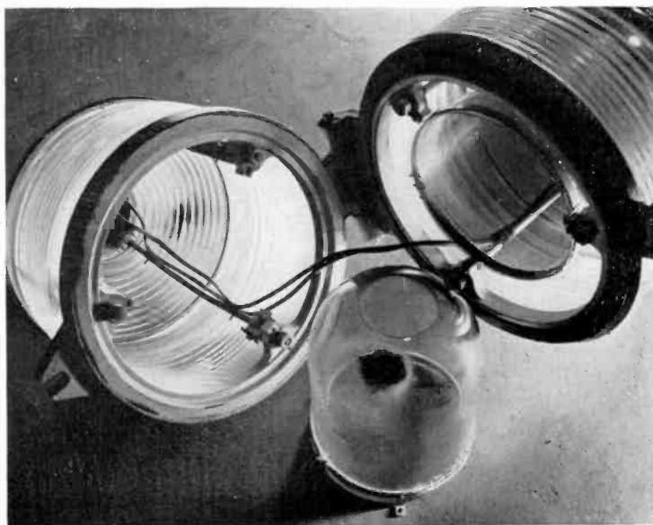
FIG. 10. The Pylon beacon as it appeared after test lightning strokes, WHEN LIGHTNING ARRESTERS WERE NOT USED. Note the wiring failure, just to the left, below the soot deposit on the left-hand lens. Also visible at the bottom of the photo is a soot deposit on the red filter.
