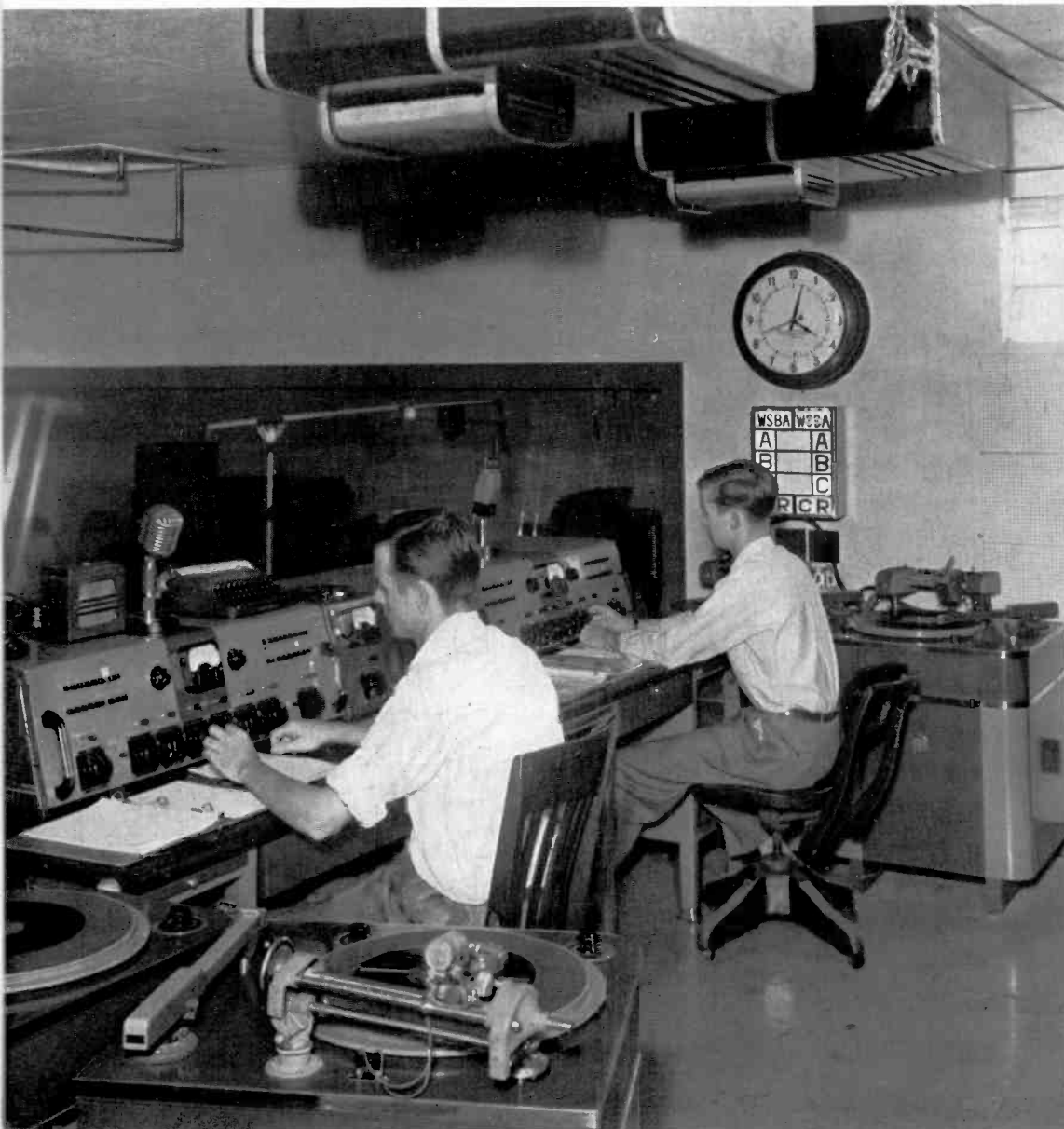
FIG. 1. (below) Complete control of studios and AM transmitter is provided by this flexible arrangement consisting of 76-B2 and 76-B4 Consolettes and 70-C2 Turntables complete with recording attachments. Messrs. Beaver and Lovett, operators, are shown at the master controls which face the AM transmitter.
