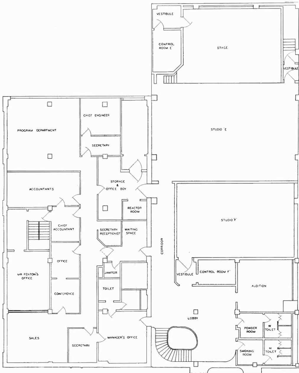
FIG. 4. (left) Arrangement of the second floor of WBAL's new installation. The "Air Theatre" and "Futuristic" studio are on this floor, as well as most of the station offices. Entry to this floor is by means of a wide circle stairway at the front of the building. The lobby is large and luxuriously furnished.
