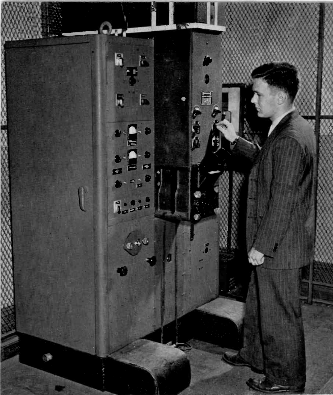
FIG. 4. In this view, an engineer is shown making observations and recording data, during tests, by means of the specially-designed cathode-ray oscillograph, or TIME MICROSCOPE, as it is sometimes called.
