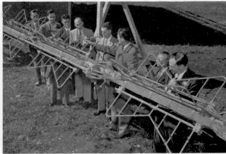
An RCA high frequency superturnstile television antenna. C. W. Armstrong, RCA engineer, is shown pointing to a broadband radiator of one of the antenna sections. Broadcasters looking on, from left to right, are: R. Craig, WCAU; Gilbert Rix, WWJ; S. E. Leonard, WTAM; F. J. Kelley, RCA; E. W. Lewis, WTVJ; J. Kyle, WMBG; W. F. Coleman, WTIC; and I. B. Robinson, The Yankee Network.
