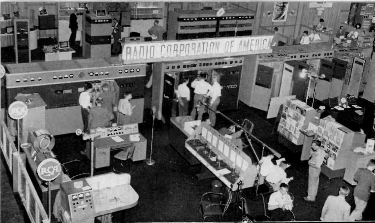
Prominent feature of the RCA booth was this line of transmitters. Left to right, the BTA-5F 5 KW AM Transmitter, the BTF-10B 10 KW FM Transmitter, and the TT-5A 5 KW TV Transmitter.
