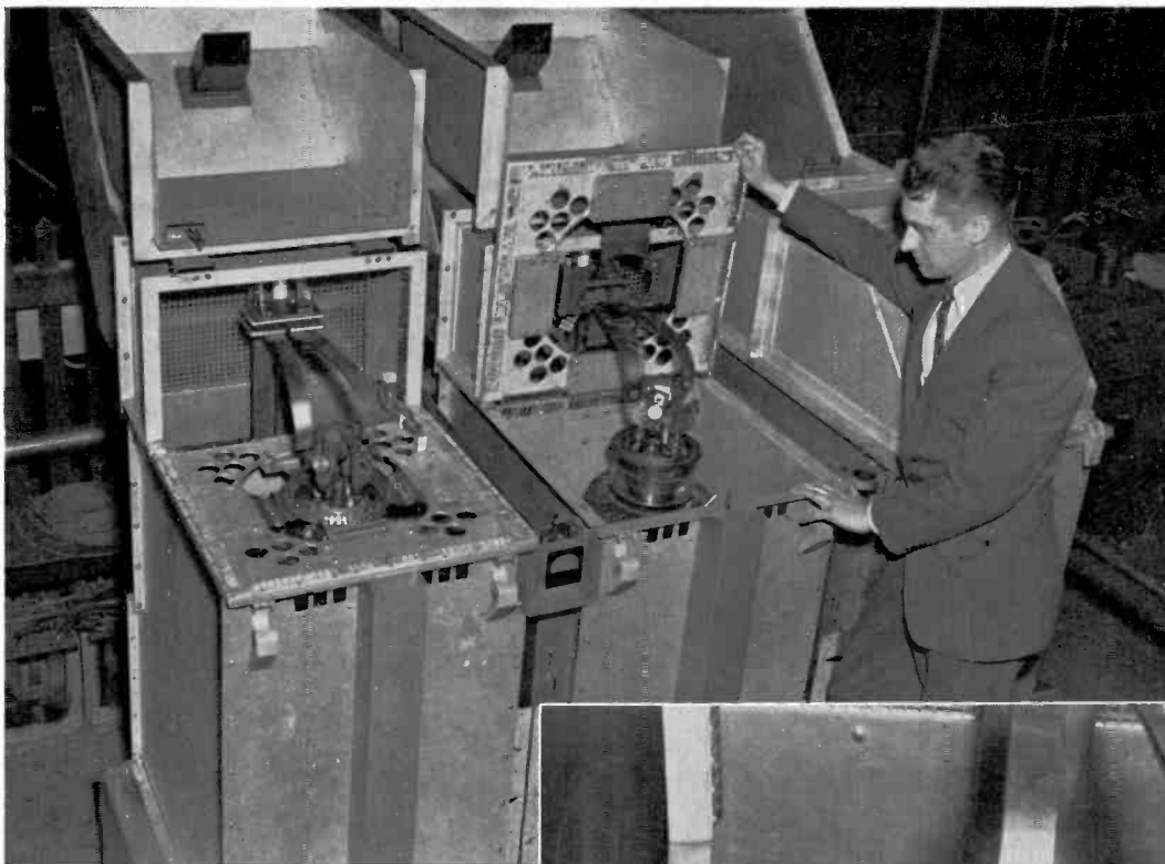
FIG. 5. (left) Another view of the 50 KW power amplifier. Dana Pratt, manager of broadcast transmitter sales, has opened two of the enclosures to show internal construction. The hood of the enclosure at the left has been raised, but the grid shield is still in place. The grid shield of the center enclosure has been lifted up to demonstrate easy access to tubes.
