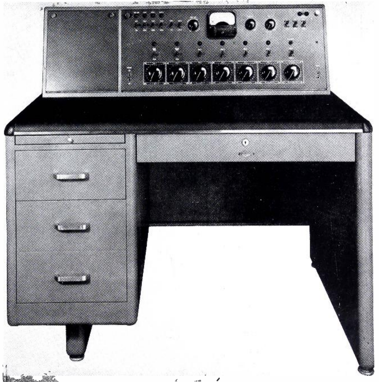
(Right) Custom-built control console used in WFAA-KGKO studio control booths. Racks which house associated amplifiers and switching equipment are shown in photo on opposite page. Schematic diagram of equipment contained in each studio setup is shown above. A converted 76-B2 Console is used in Studio D control booth.
